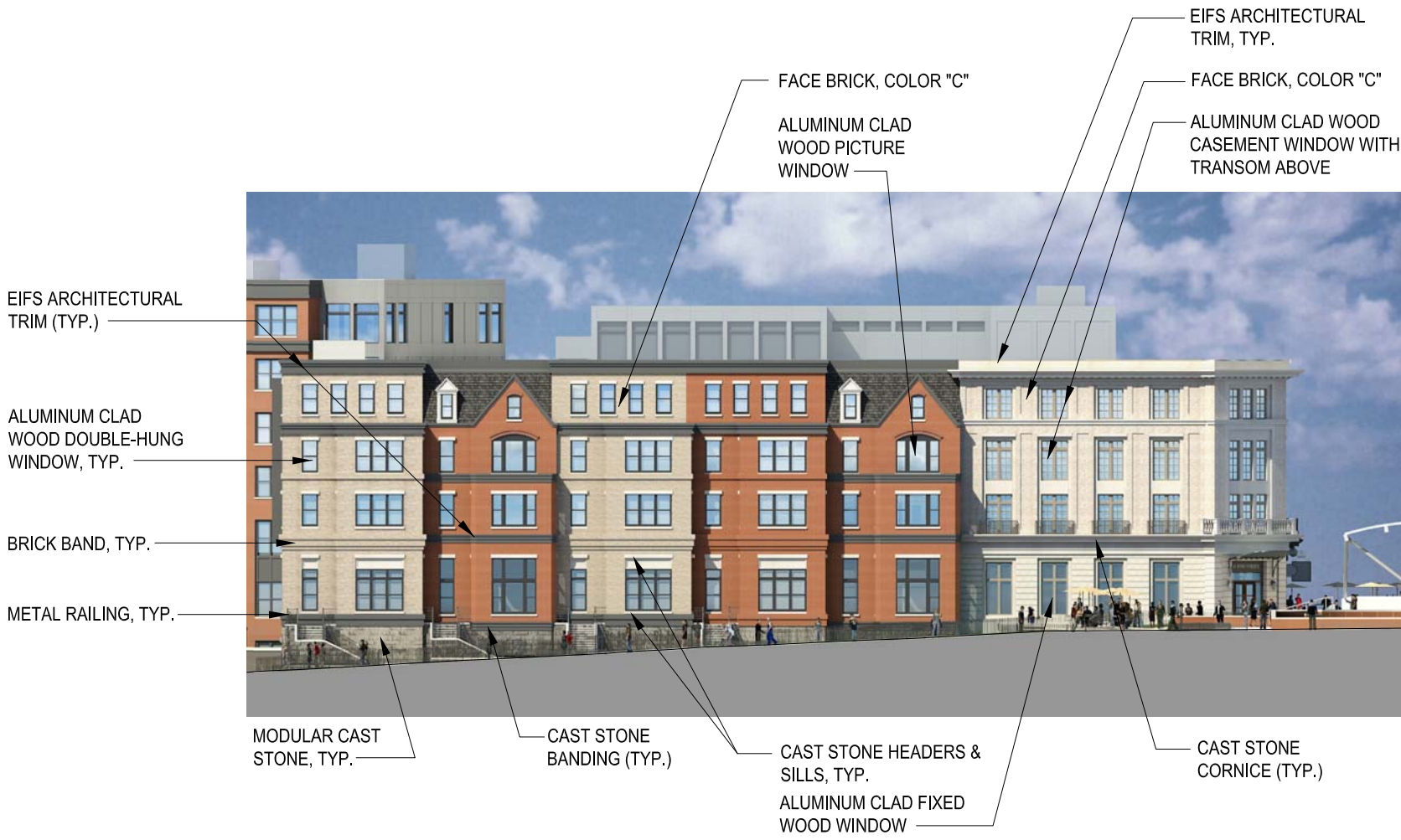
2 C STREET ELEVATION (SECONDARY STREET) Scale: 1/32" = 1'-0"
