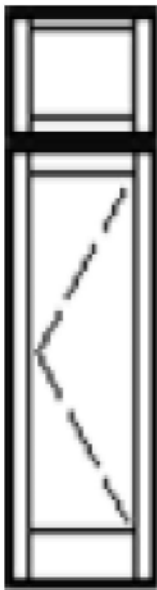
08 FRAME SIZE: 37 5/8 X 106 1/2, BTM = 82 1/2 SITELINE CLAD AURALAST PINE, INSWING DOOR PRODUCT, (SINGLE-SWING) SINGLE DOOR WITH 1 TRANSOM, (LEFT), BTM=82 1/2, 4 5/8" STILE, 8 1/4" BOTTOM RAIL, BLACK EXTERIOR, CLEAR FRAME SATIN NICKEL HINGE, INSULATED LOW -E 366 PRESERVE FILM
