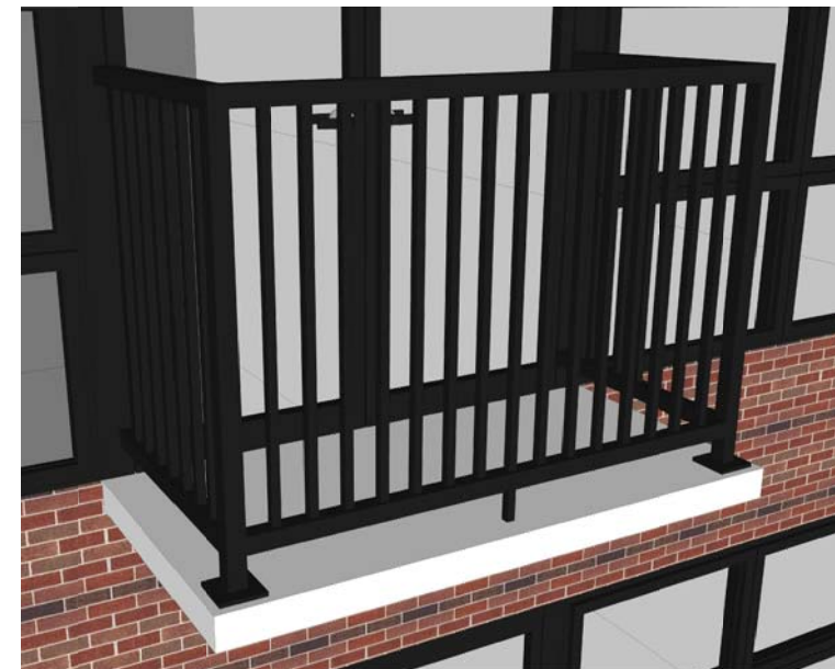
14 CONCRETE DECK ON WHITE EPOXY PAINT FINISH
