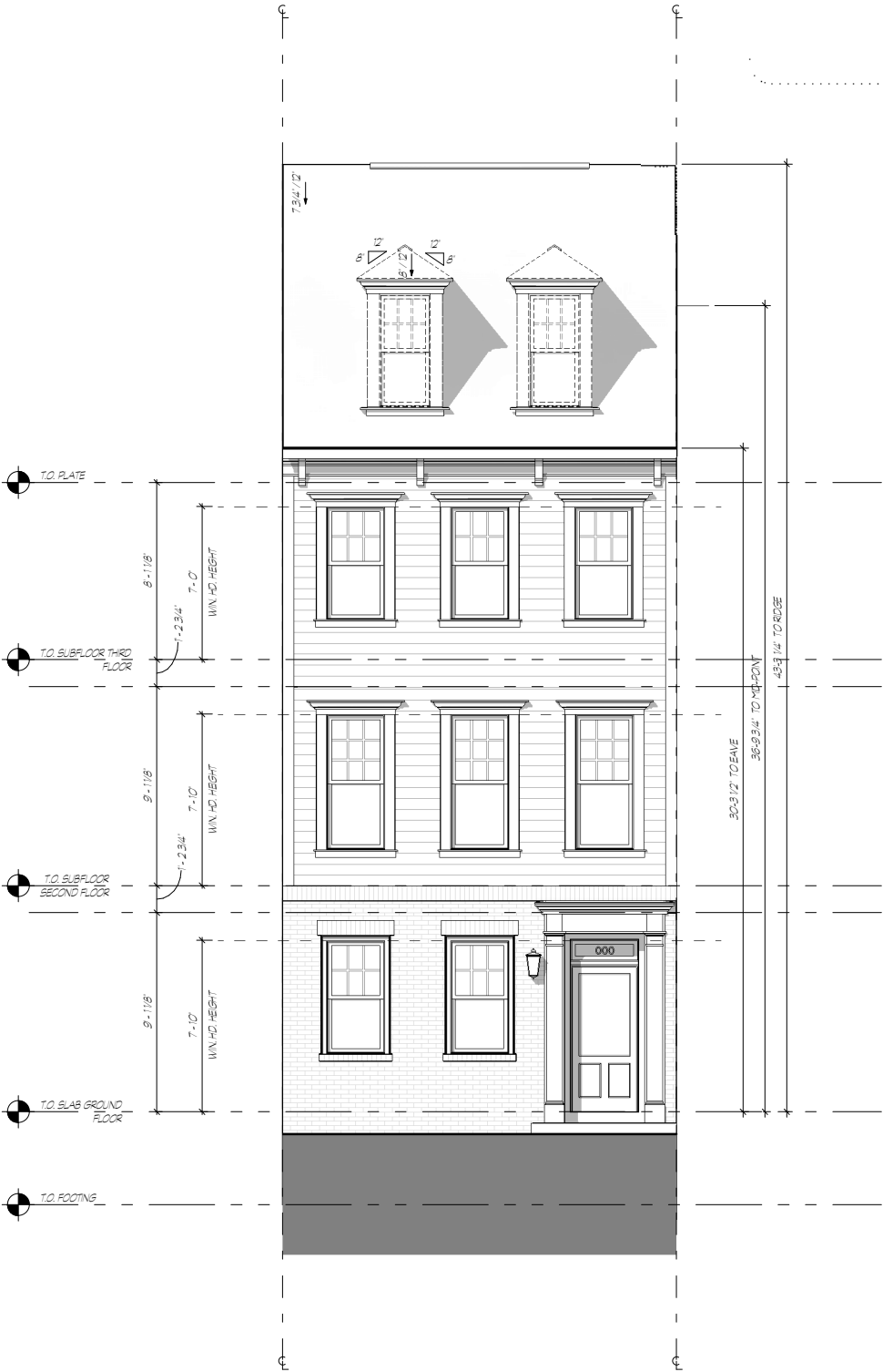
1 FRONT ELEVATION D - BRICK WATER TABLE
