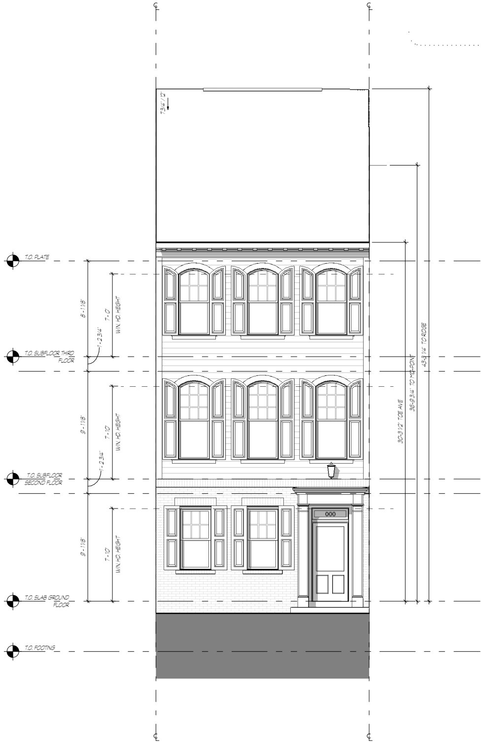
1 FRONT ELEVATION C - BRICK WATER TABLE
