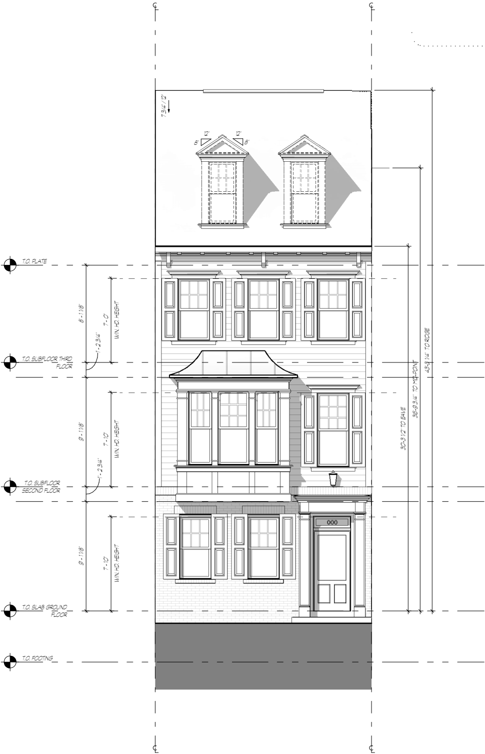
1 FRONT ELEVATION B - BRICK WATER TABLE
