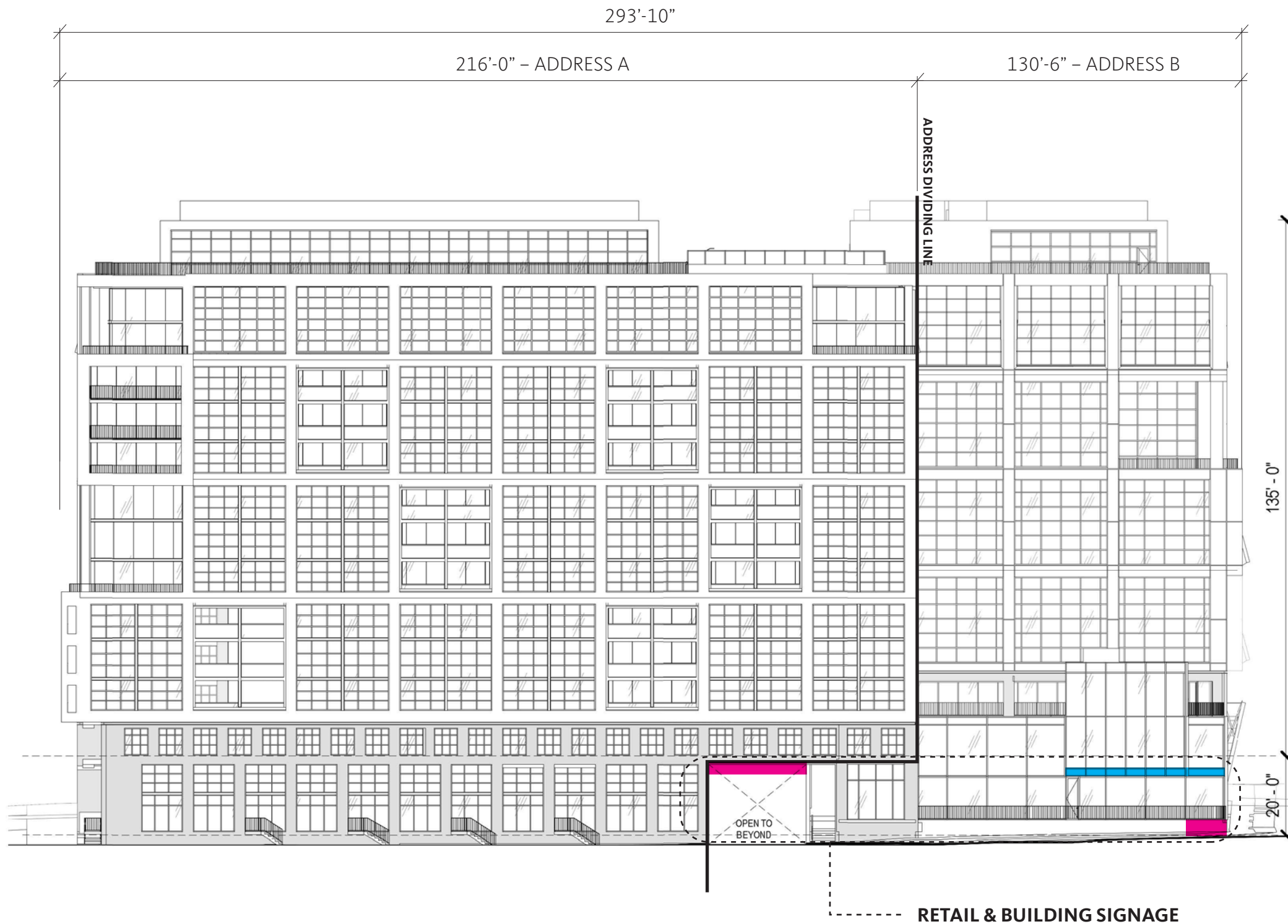
1 ELEVATION: WEST SCALE: 1"=30'-0"
