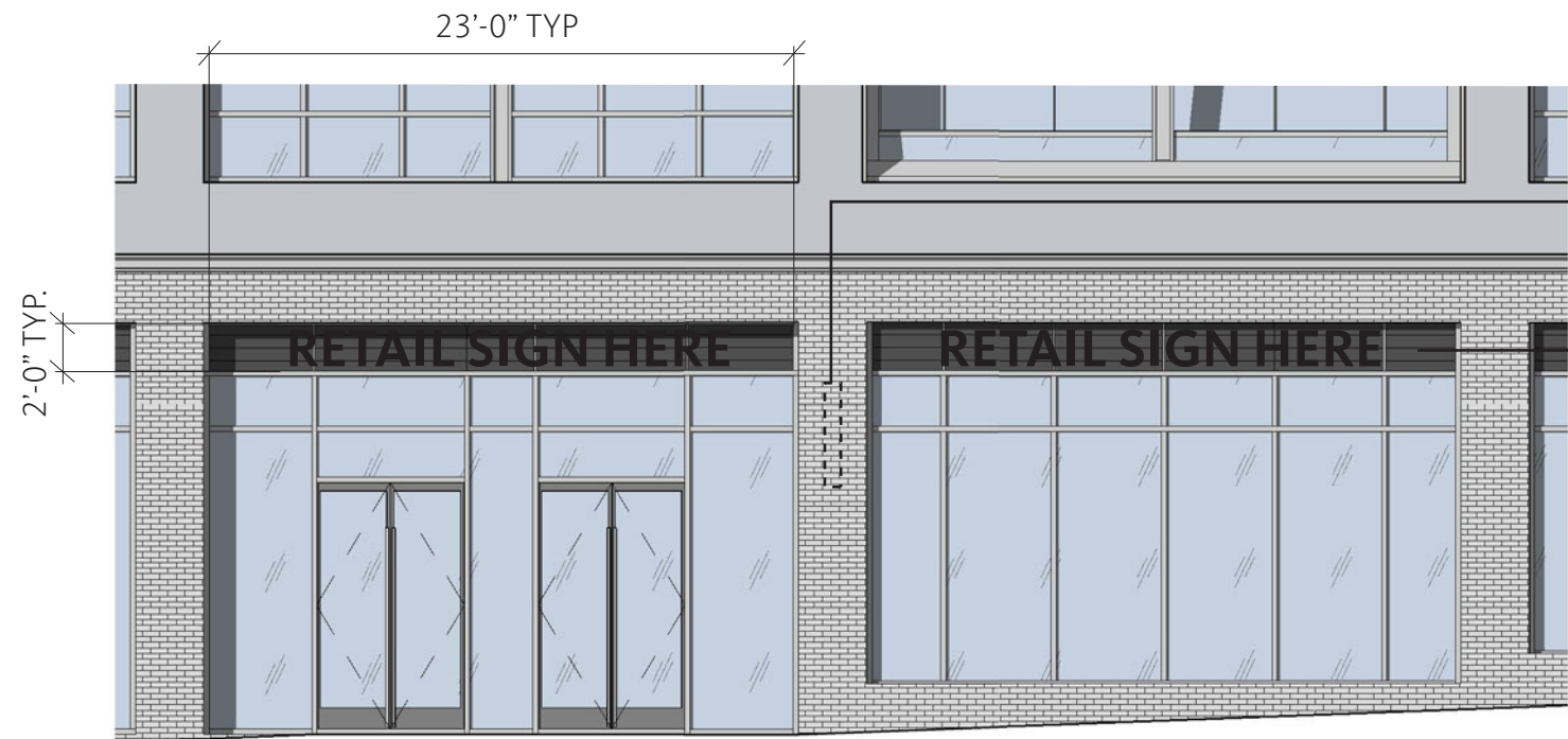
1 TYPICAL STOREFRONT DETAIL SCALE: 1/2"=1'-0"
