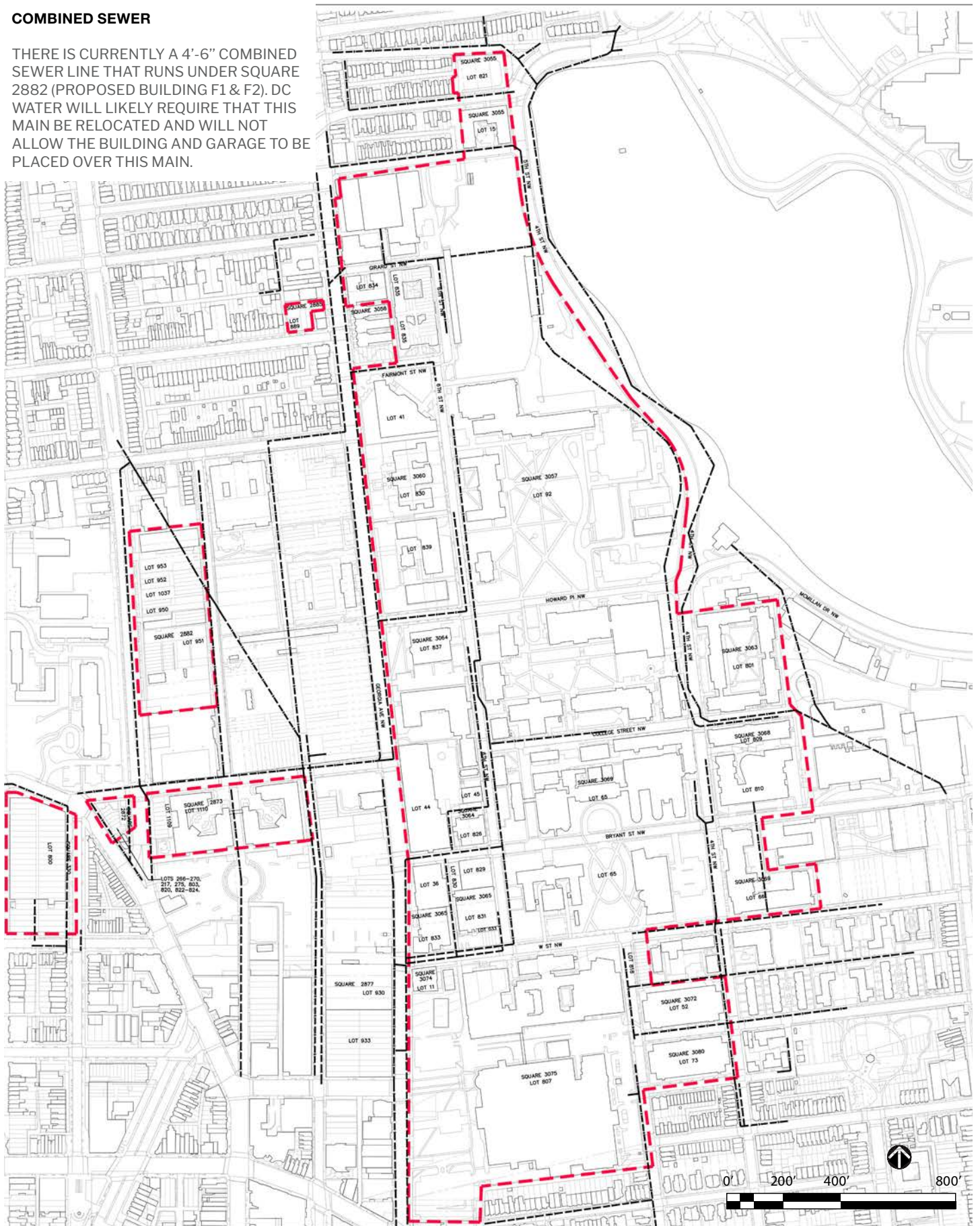
Figure 3.34: Combined Sewer Distribution
