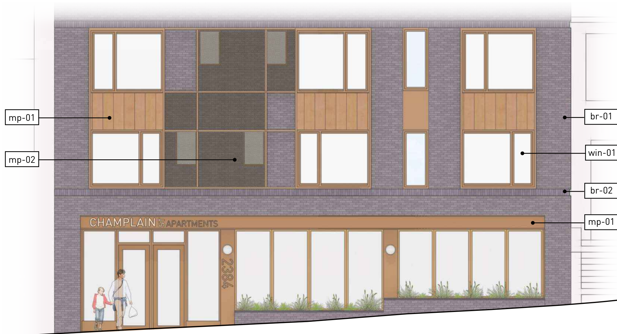
br-01 face brick dark ironspot smooth norman size charcoal mortar
