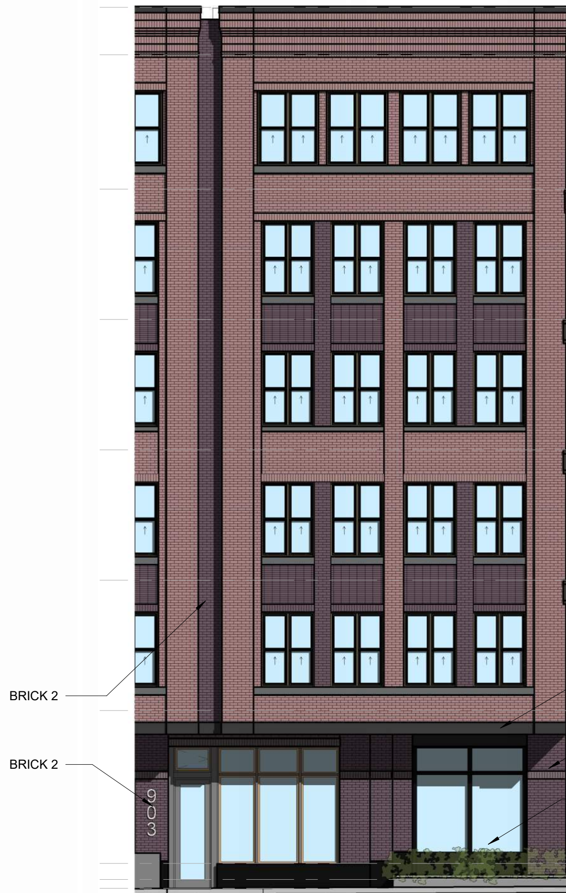
② North Elevation - Typical Bay of Live/Work Units 1/8" = 1'-0"
