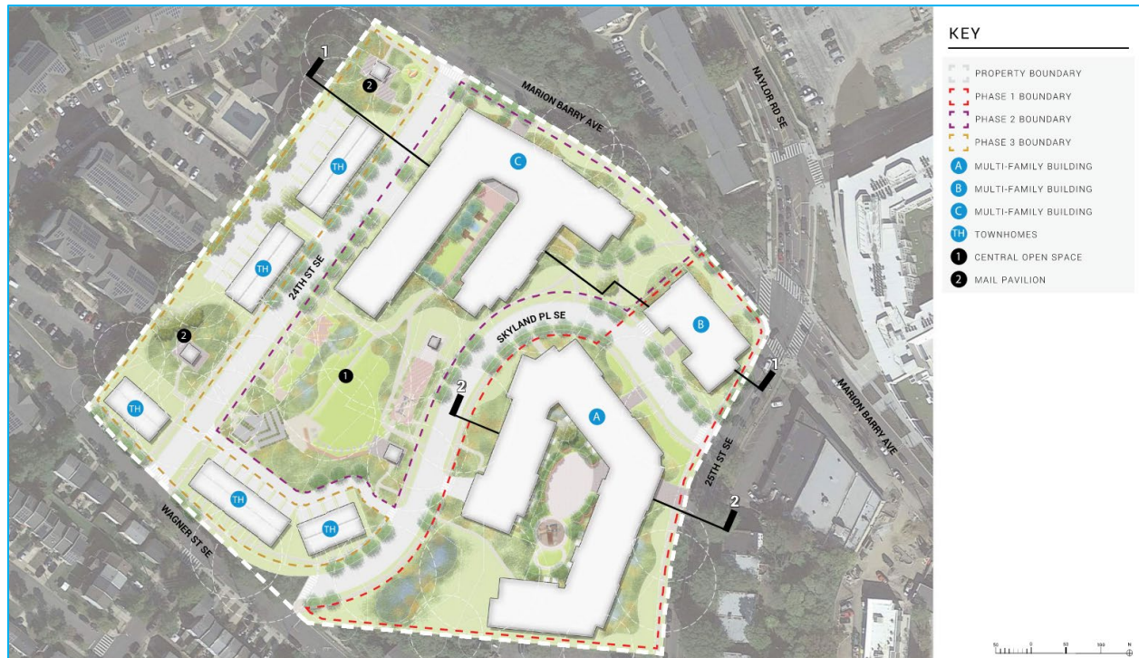
Figure 2: Proposed Phasing Plan.
