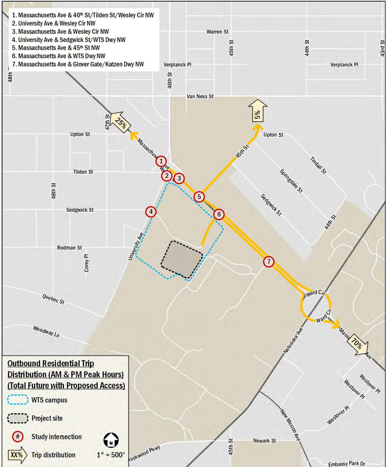
Figure 16: Outbound Trip Distribution (Total Future with Proposed Access: w/ University Ave Driveway Exit Restricted During Peak Periods – Delivery Vehicle Access Maintained)
