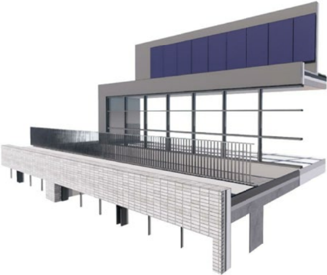
Vertical solar panels
