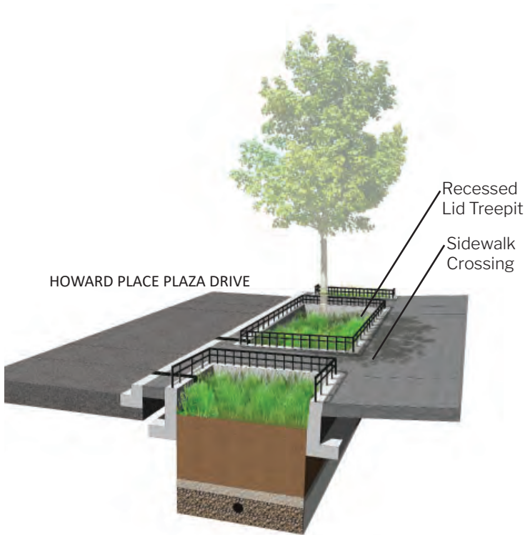
Figure 4.62: Tree Pit Bioretention
