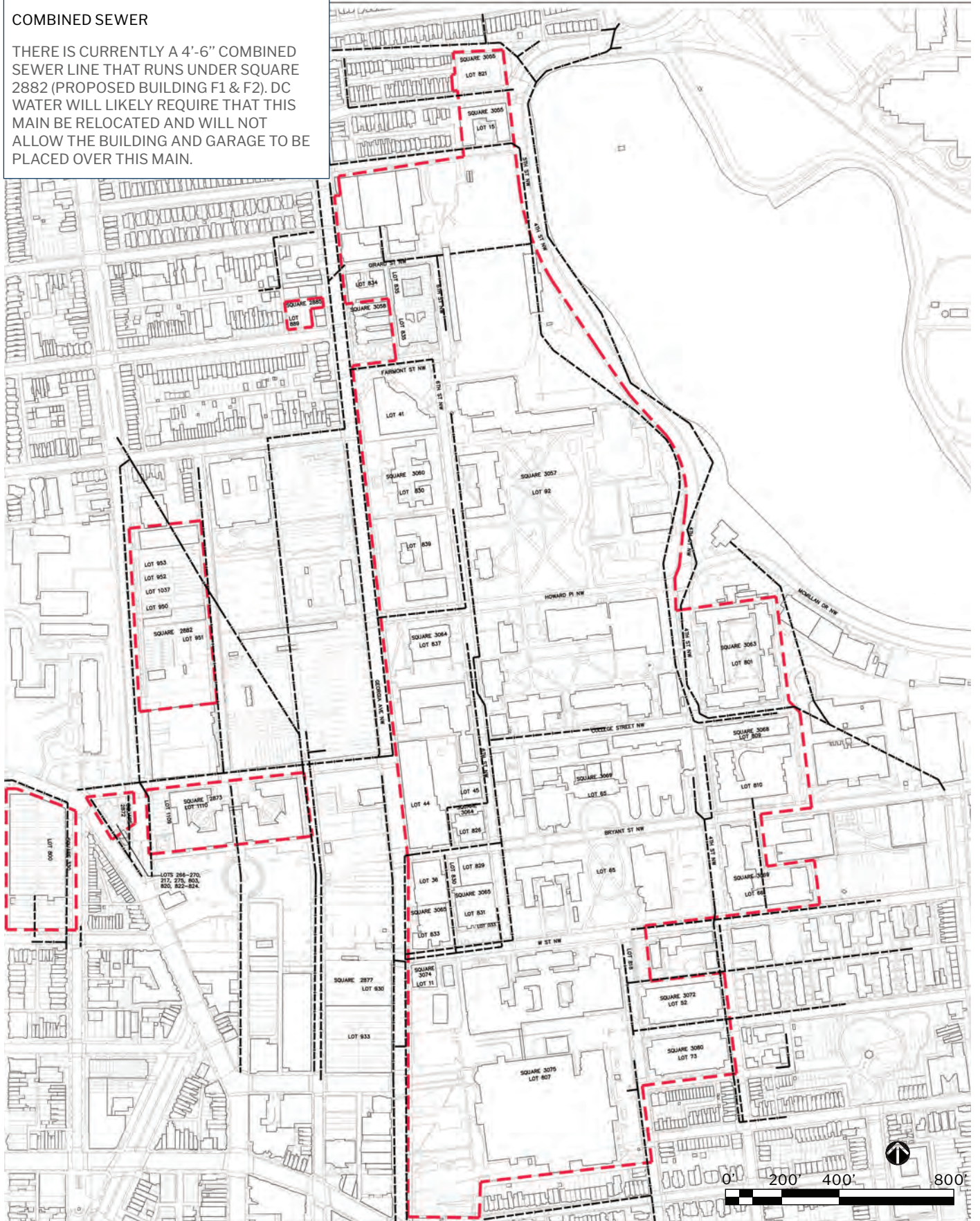
Figure 3.33: Existing Combined Sewer Distribution
