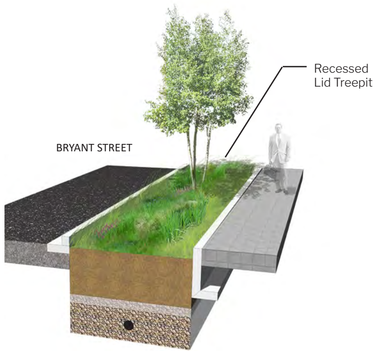
Figure 4.66: Continuous Tree Pit - Lid Planter
