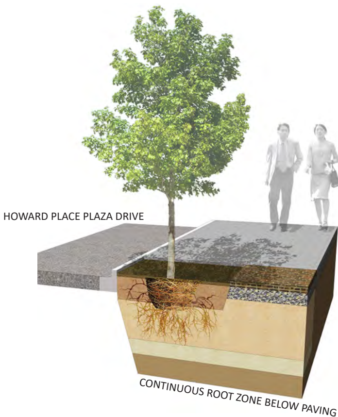
Figure 4.63: Continuous Tree Pit
