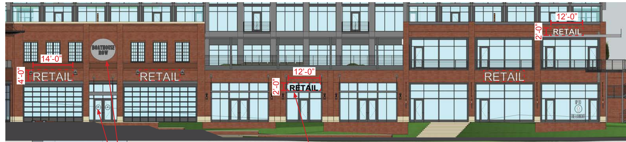
② Lower Retail Plaza Halo Lit Metal Building Signage Mounted on Metal Surface Internally Illuminated Acrylic Signage TBD by Retail Tenant Window Vinyl Decal Graphic
