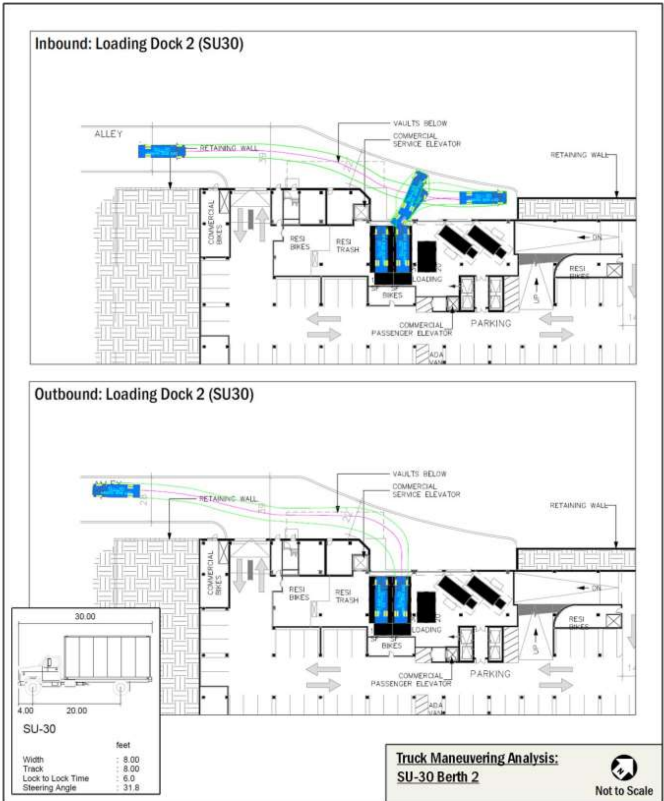
Figure 15: Truck Maneuvering Analysis: SU-30 Berth 2
