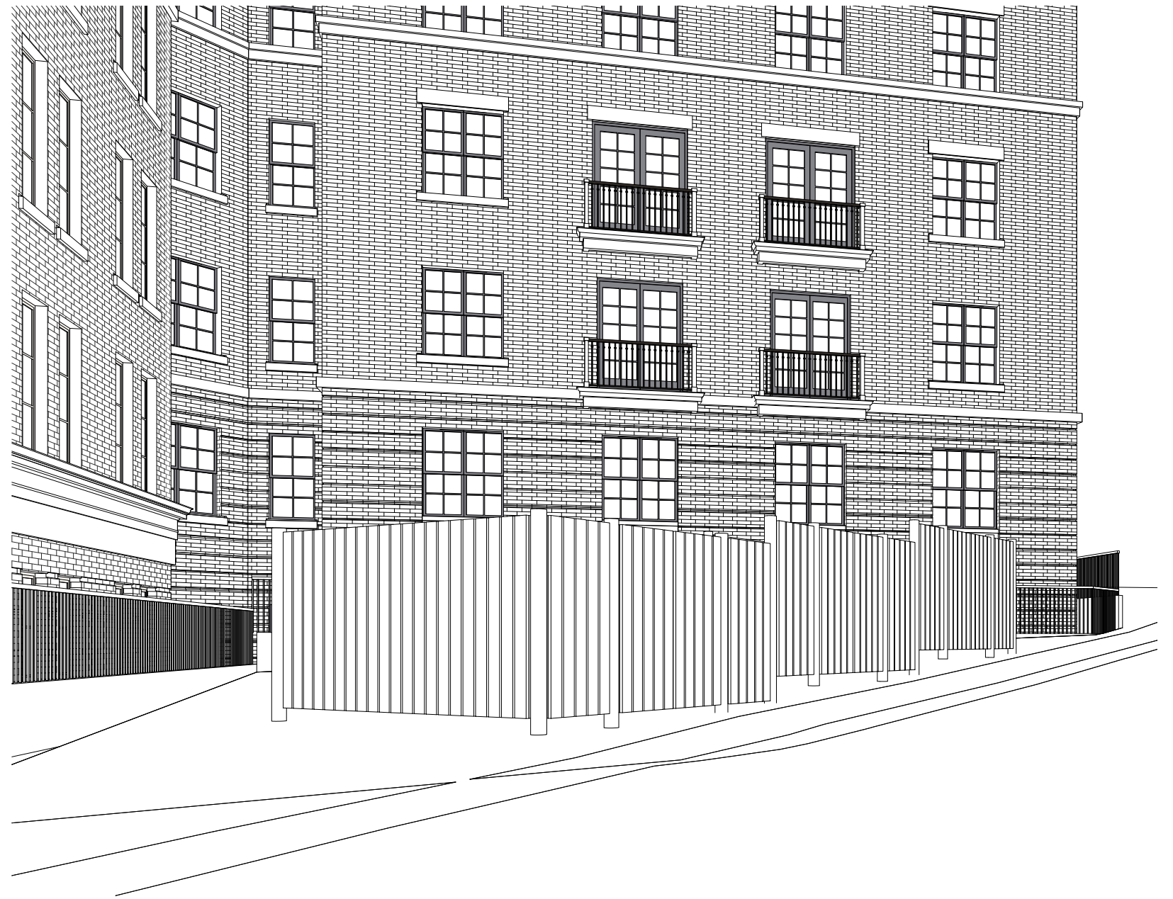
VIEW FROM ALLEY SHOWING SCREENING FOR TRANSFORMERS
