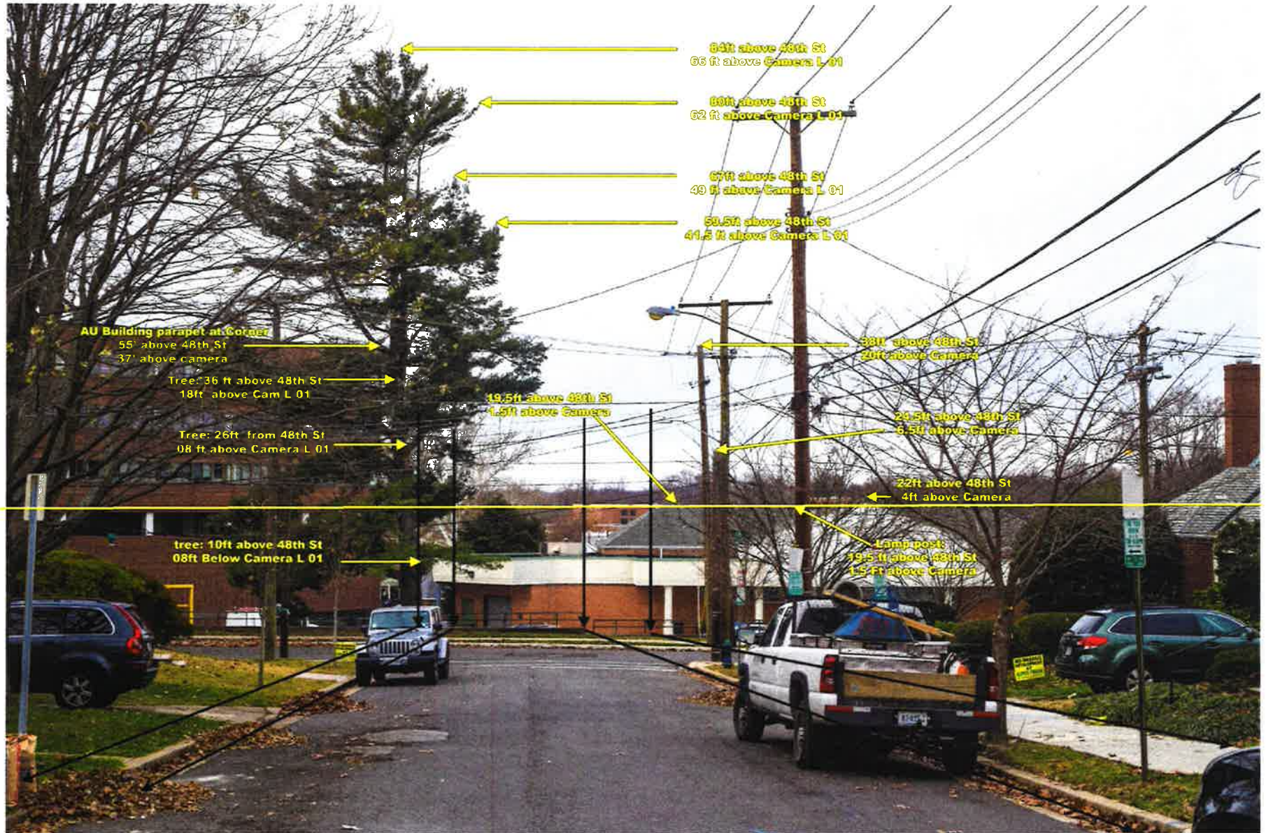
Laser measurements of the existing structures were taken to use as references. These fixed objects were used when verifying the 3D model's placement and scaling. www.AirPhotosLIVE.com
