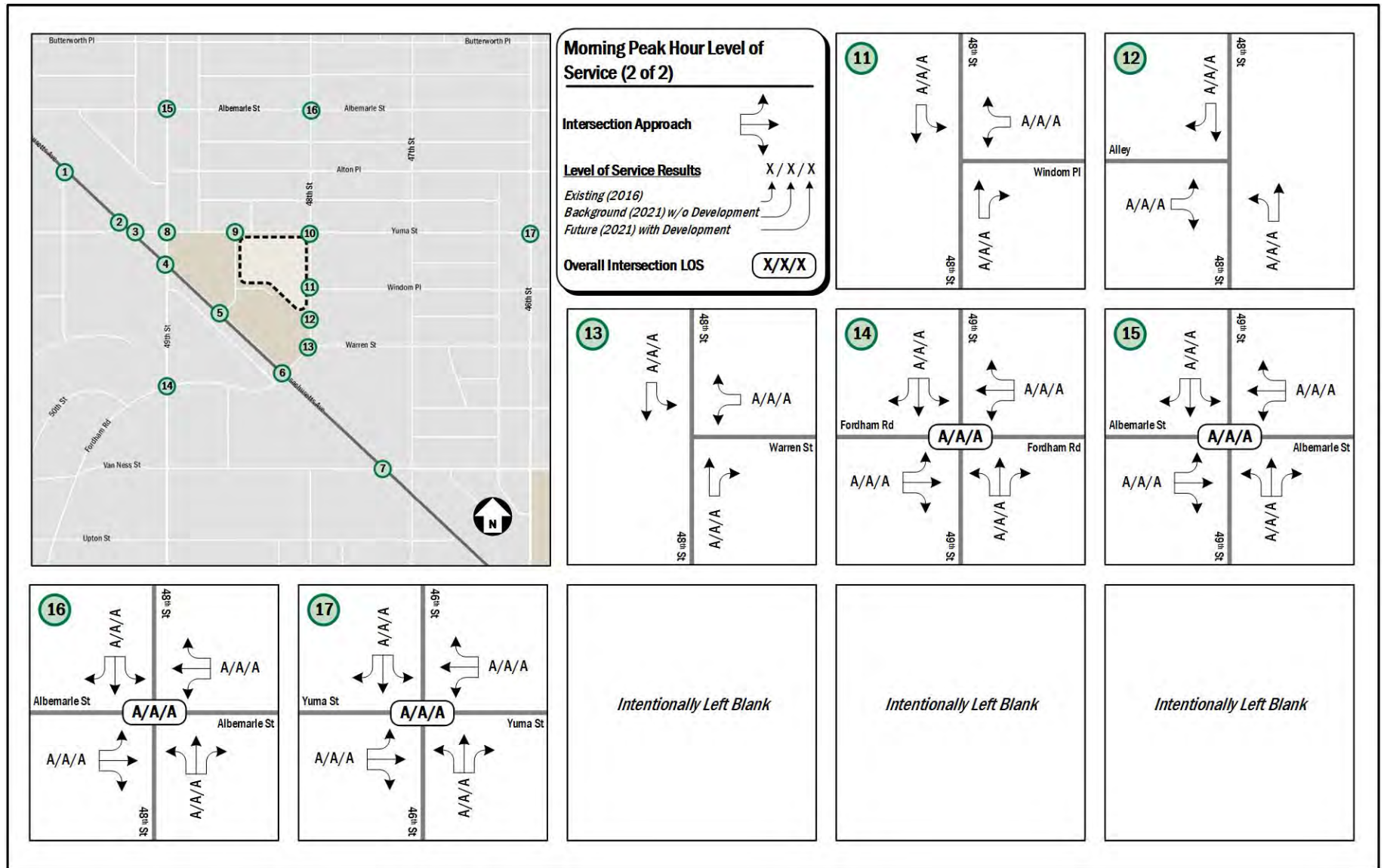
Figure 28: Morning Peak Hour Capacity Analysis Results (2 of 2)
