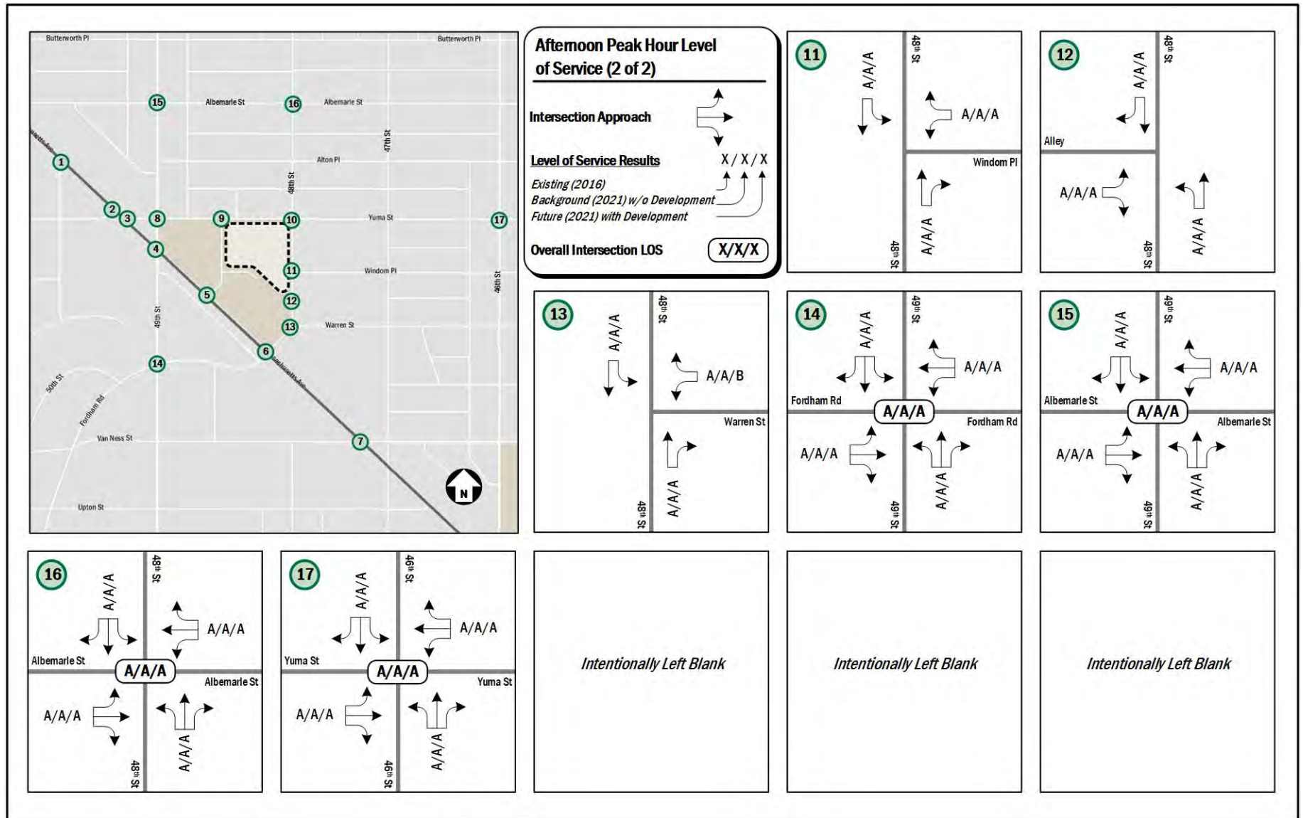
Figure 30: Afternoon Peak Hour Capacity Analysis Results (2 of 2)
