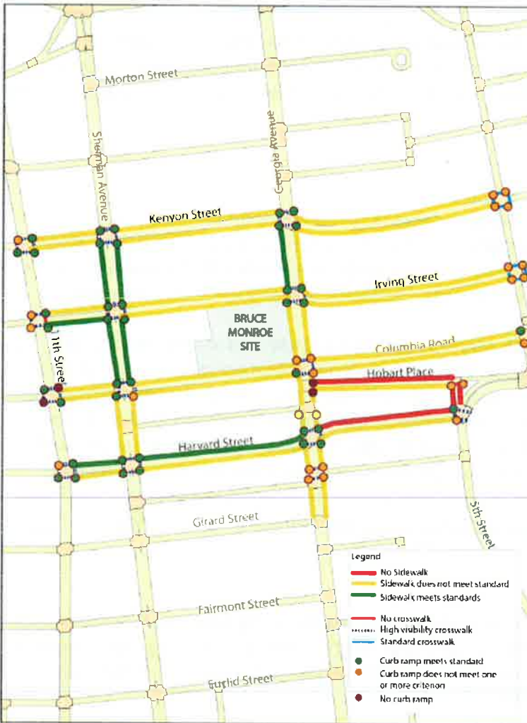
Figure 4 Existing Pedestrian Facilities Inventory
