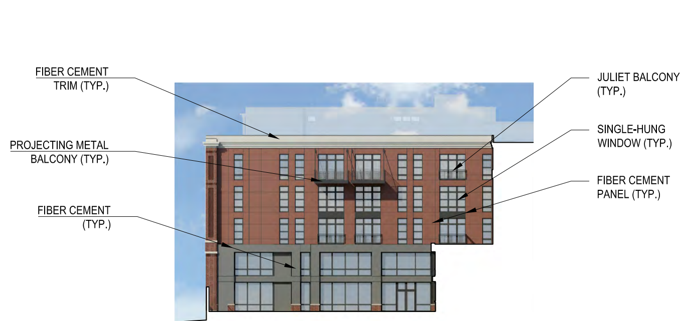
1 F1 COURTYARD ELEVATION LOOKING SOUTH Scale: 1/32" = 1'-0"
