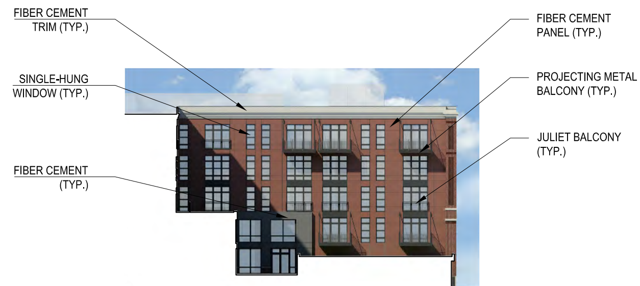
3 F1 COURTYARD ELEVATION LOOKING NORTH Scale: 1/32" = 1'-0"
