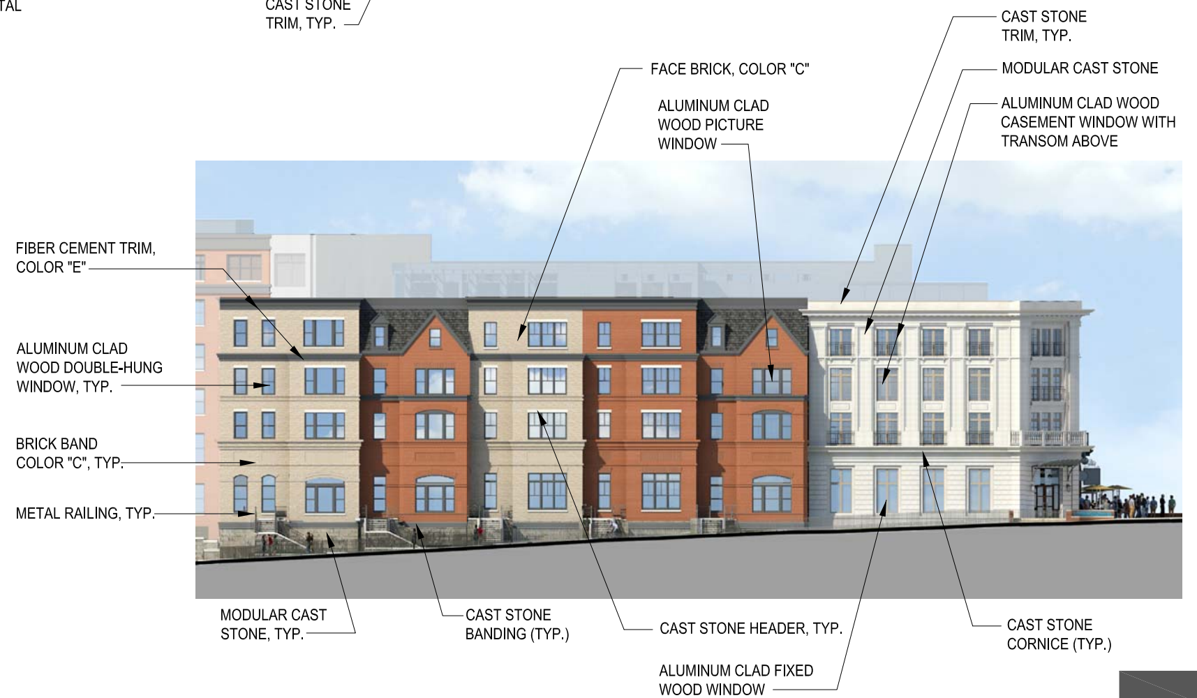
3 C STREET ELEVATION (SECONDARY STREET) Scale: 1/32" = 1'-0"
