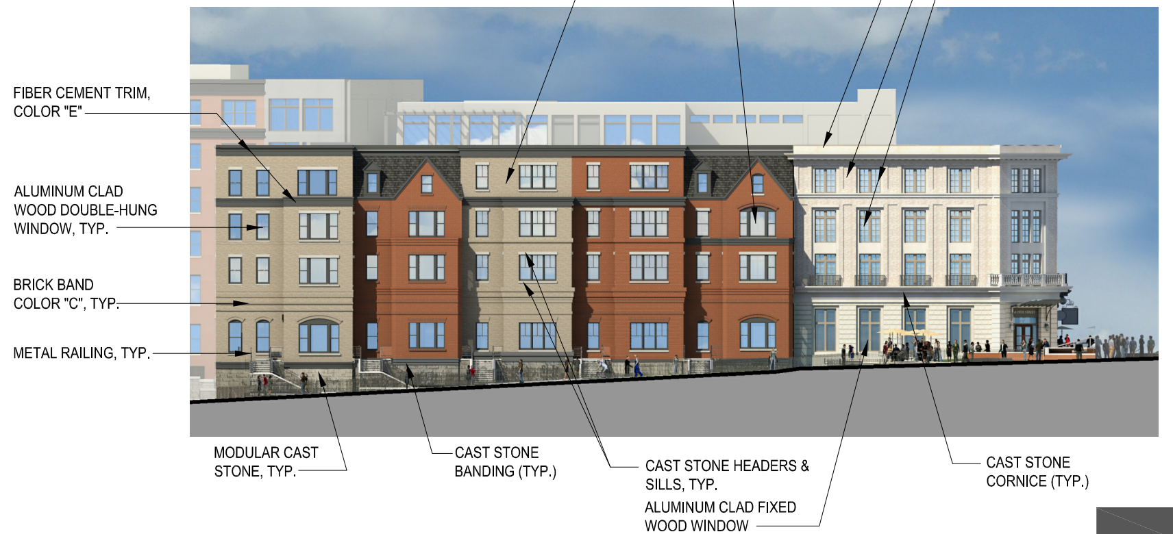
3 C STREET ELEVATION (SECONDARY STREET) Scale: 1/32" = 1'-0"
