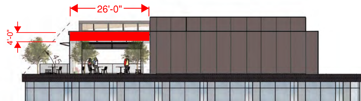
POTENTIAL SIGNAGE LOCATIONS - SOUTH PENTHOUSE ELEVATION
