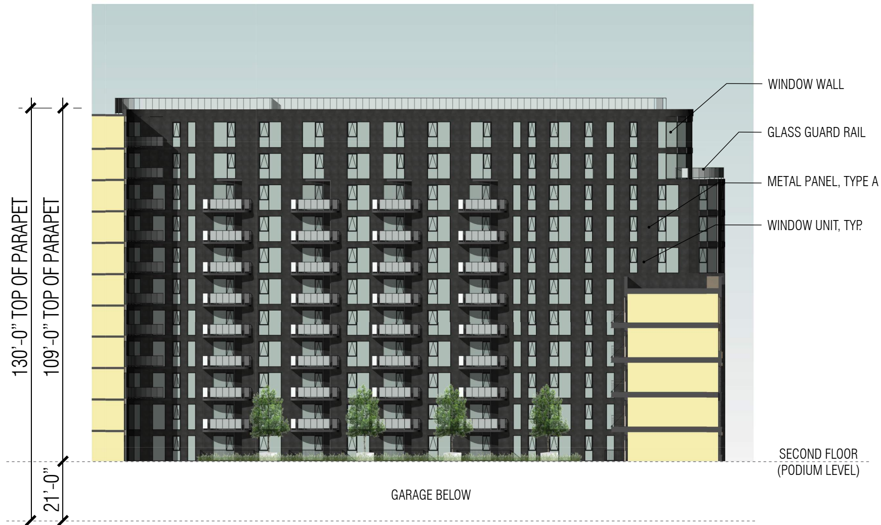
2 – COURTYARD WEST ELEVATION
