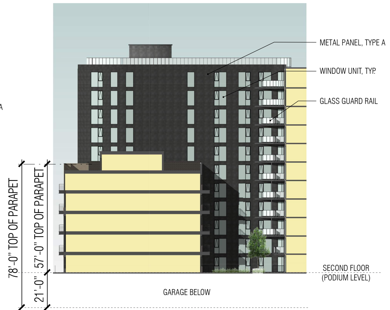
1 – COURTYARD NORTH ELEVATION
