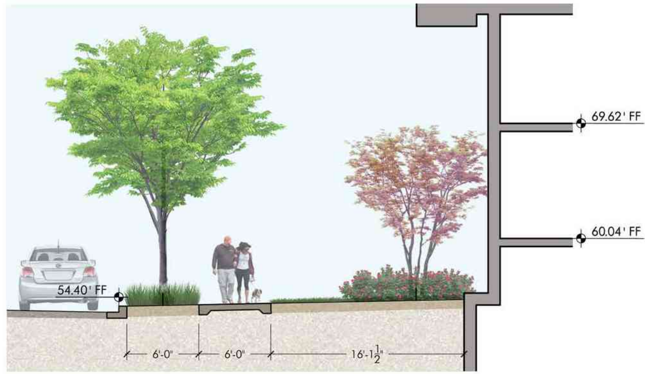
SECTION 1 - 1ST STREET NW SCALE: 1/8"=1'-0"
