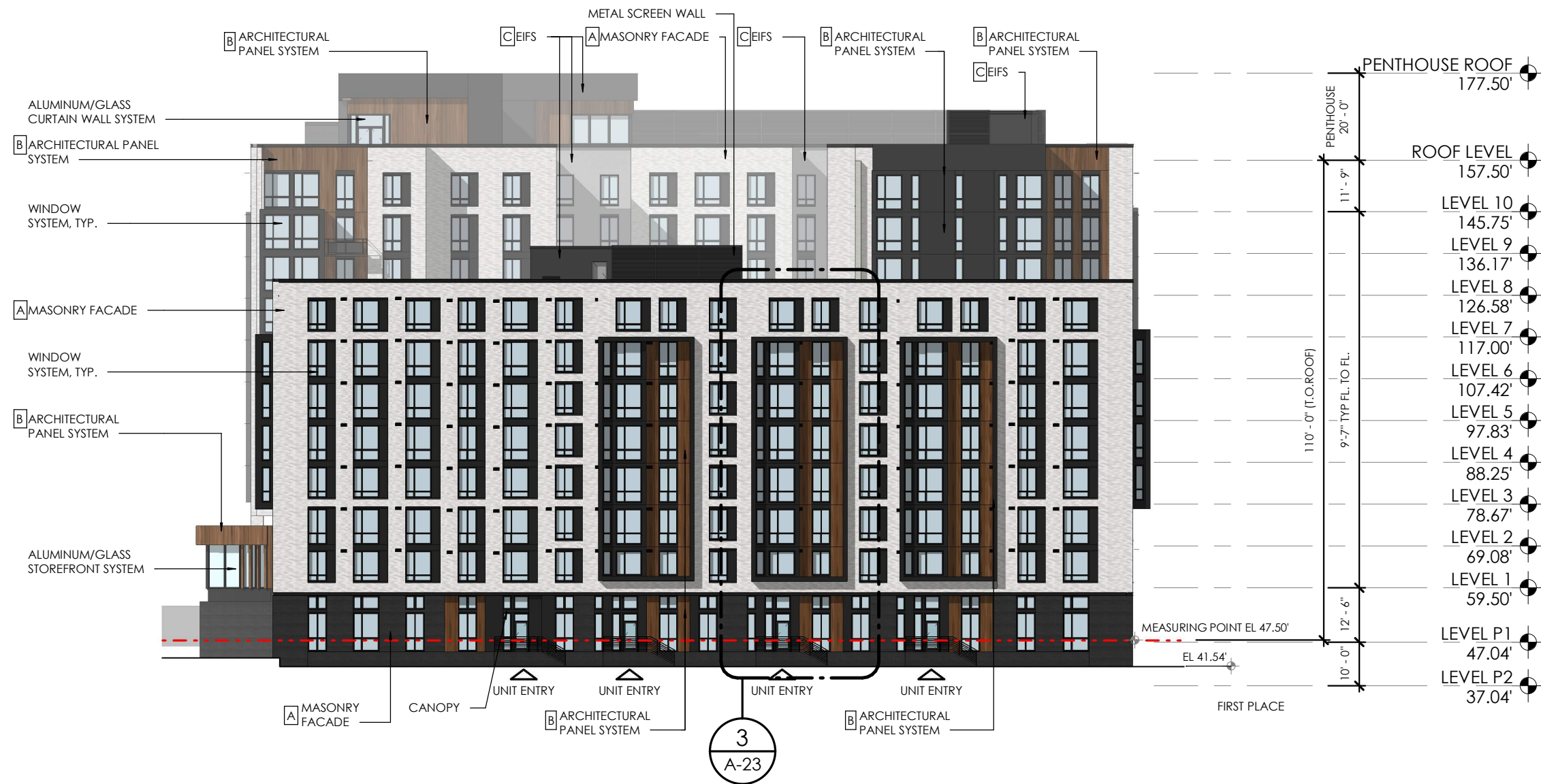
SOUTHEAST BUILDING - SOUTH ELEVATION
