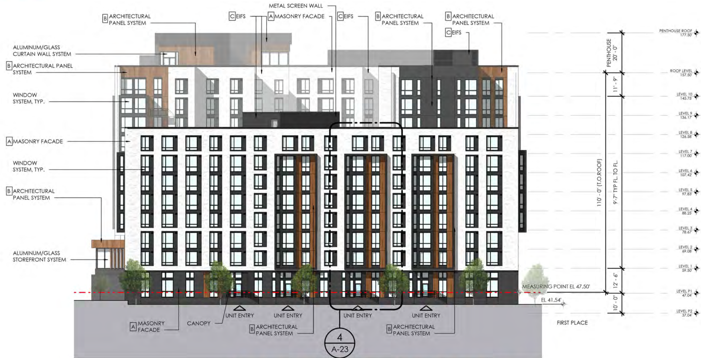
SOUTHEAST BUILDING - SOUTH ELEVATION
