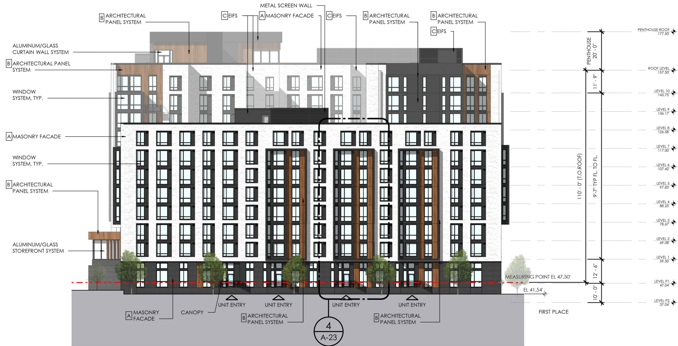
SOUTHEAST BUILDING - SOUTH ELEVATION
