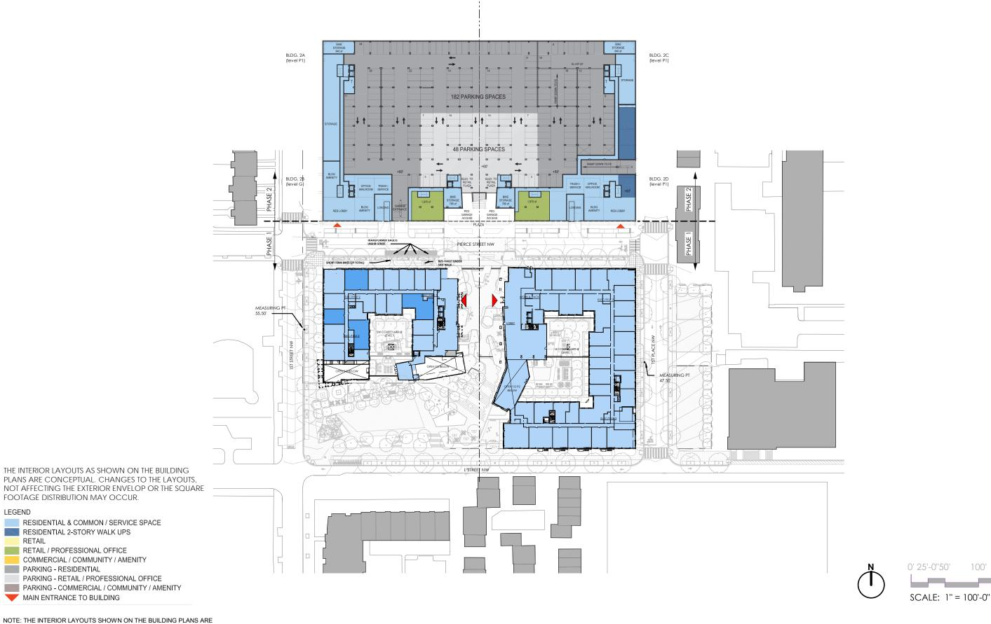
Proposed Ground Floor (Phase 1) & Level P1 (Phase 2) Floor Plans
