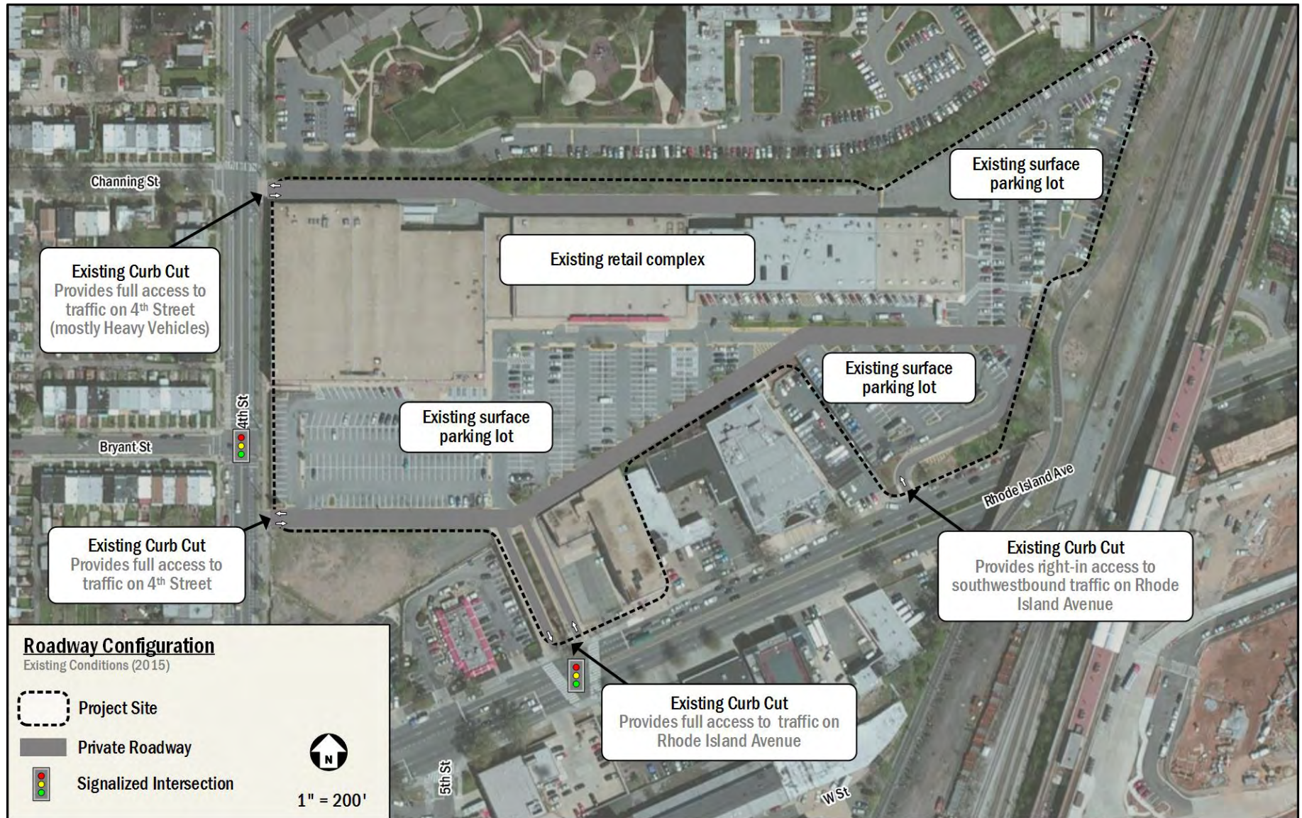
Figure 11: Existing Roadway Configuration
