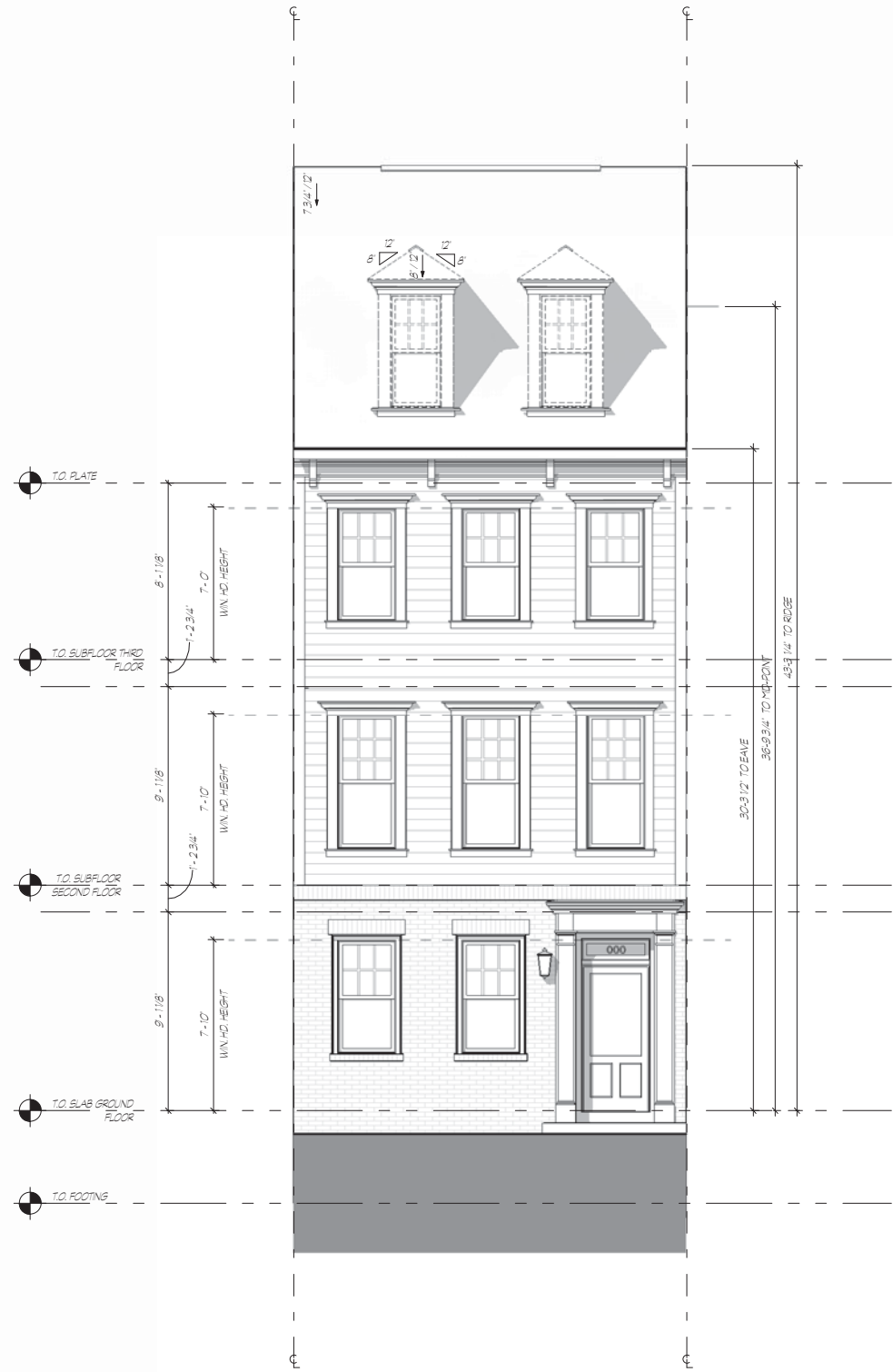
1 FRONT ELEVATION D - BRICK WATER TABLE
