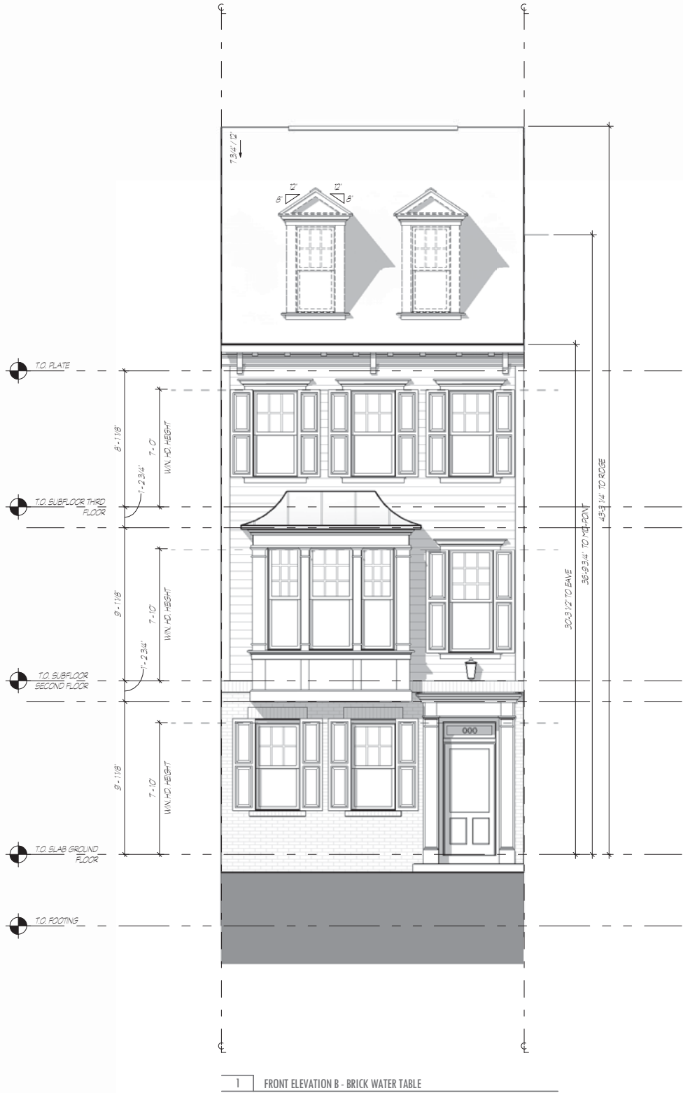
1 FRONT ELEVATION B - BRICK WATER TABLE
