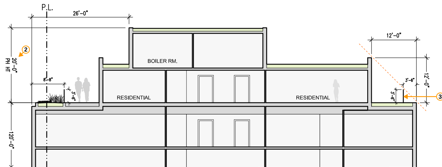
Ⓑ - SOUTH / NORTH ROOFTOP SECTION
