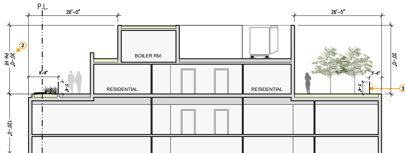
Ⓑ - SOUTH / NORTH ROOFTOP SECTION
