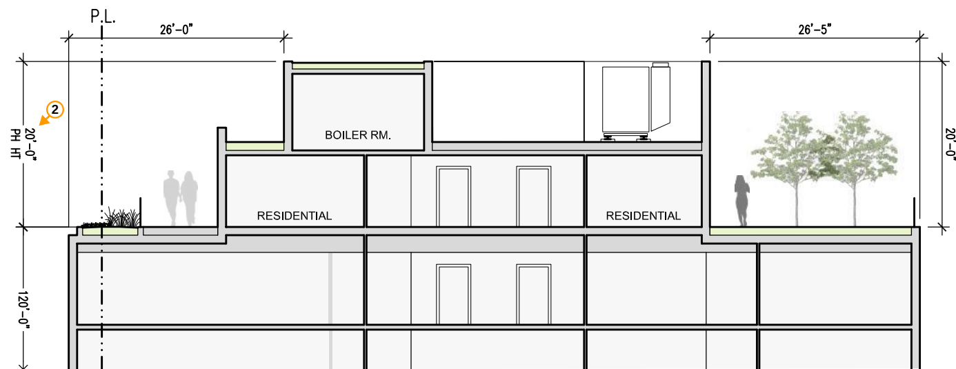
Ⓑ - SOUTH / NORTH ROOFTOP SECTION
