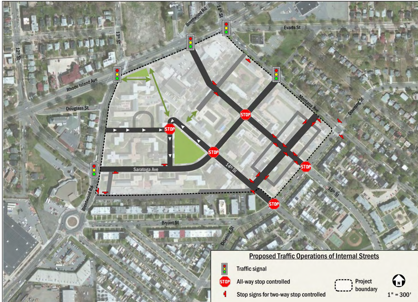
Figure 29: Traffic Operations of Internal Roadways
