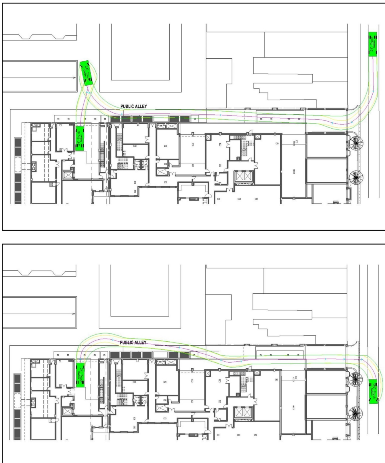
Figure 8: 24' Delivery Truck Turning Movement Diagrams – West Residential Loading Bay
