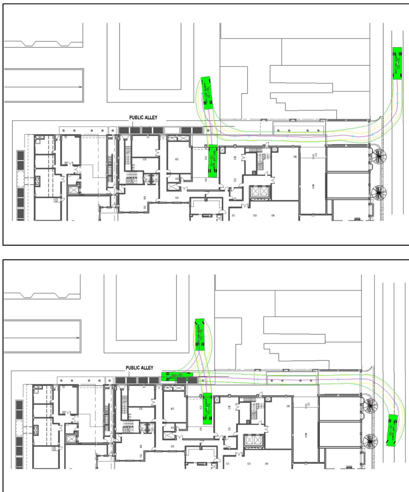
Figure 11: SU-30 Turning Movement Diagrams – East Hotel Loading Bay
