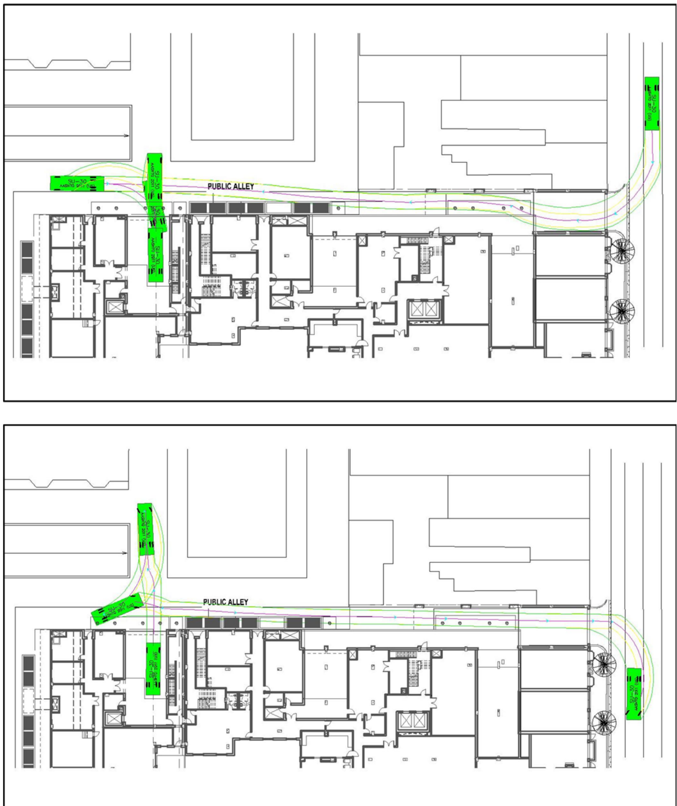
Figure 9: SU-30 Turning Movement Diagrams – East Residential Loading Bay
