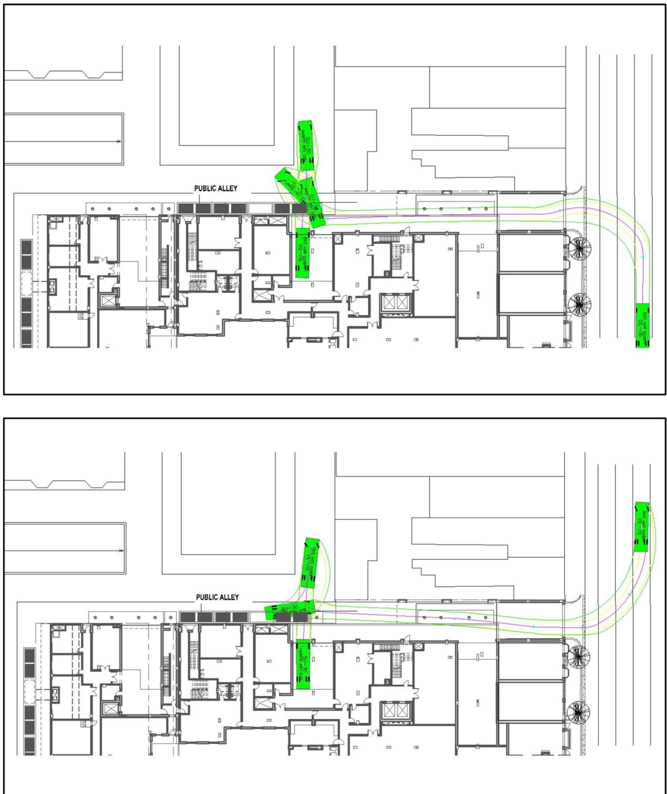
Figure 10: SU-30 Turning Movement Diagrams – West Hotel Loading Bay
