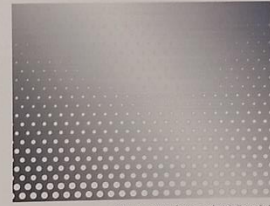
1. Metal Panel Pattern: Panels are perforated with a gradient of round holes that vary from 1/4" in diameter to 3/4" in diameter.
