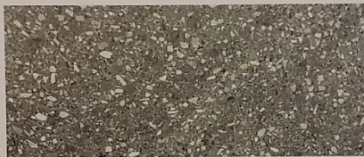
3. Ground Face Block: Visible structural block will have a dark ground-face finish.
