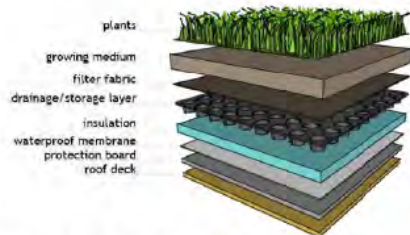
TYPICAL DETAILS FOR GREEN ROOF ASSEMBLY
