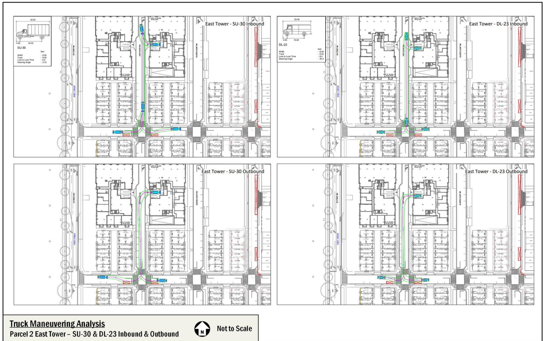
Figure 9: Truck Turning Maneuvering Analysis – Parcel 2 East Tower – SU-30 & DL-23 Inbound & Outbound
