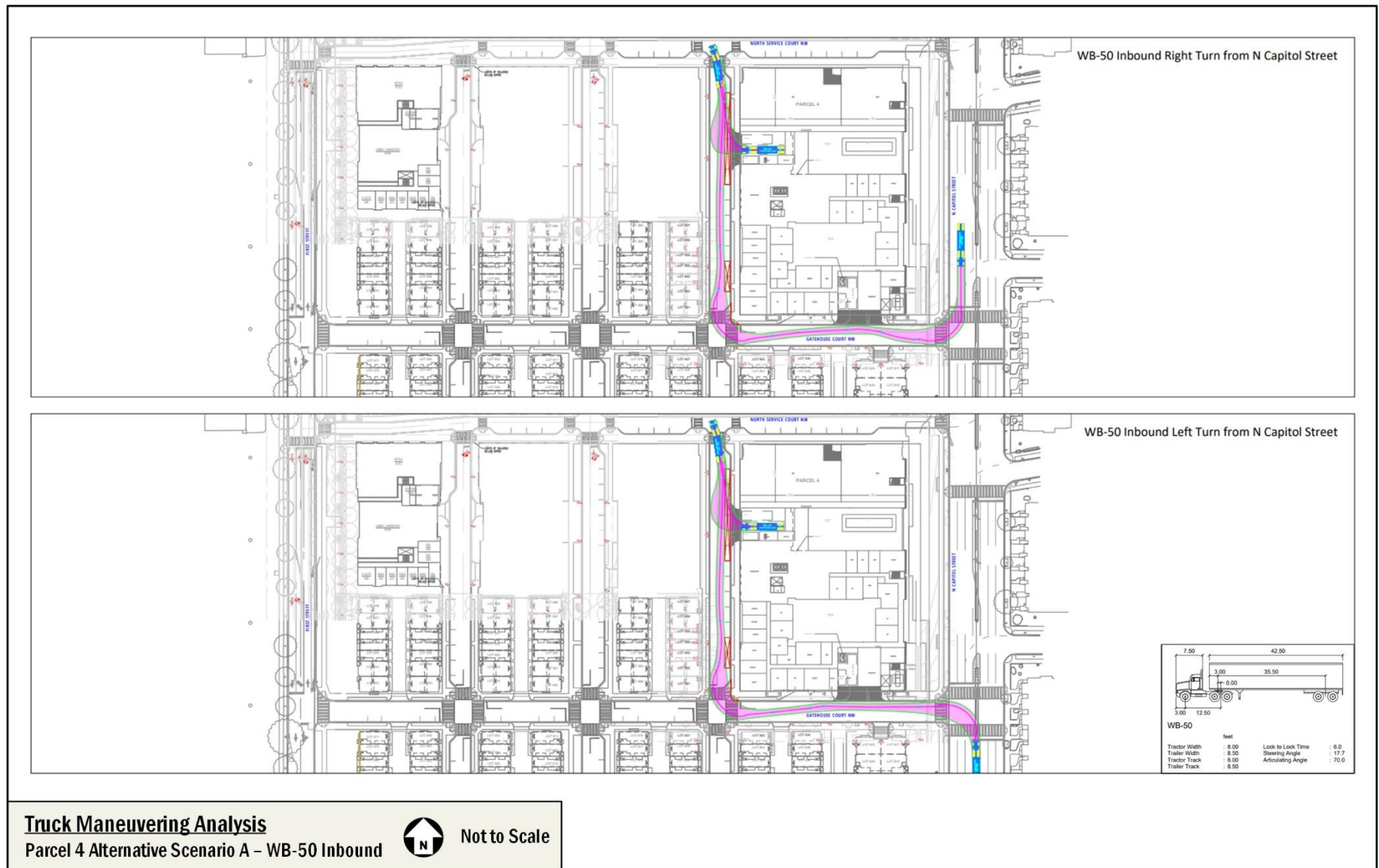
Figure 13: Truck Maneuvering Analysis – Parcel 4 Alternative Scenario A – WB-50 Inbound
