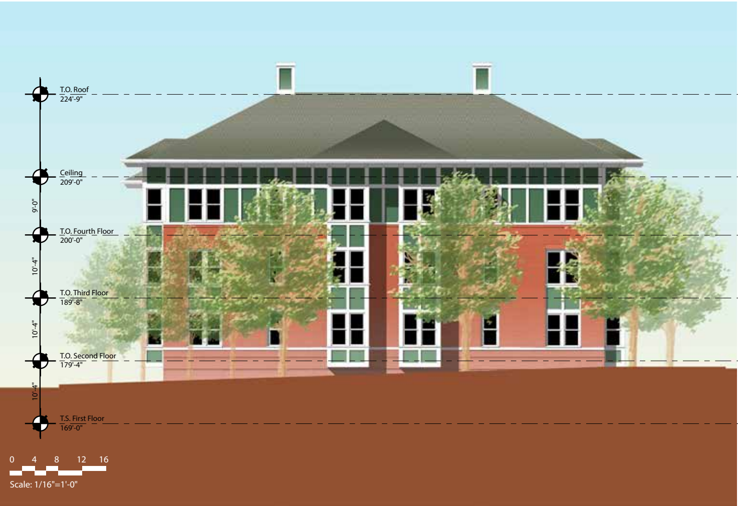
Building B North Elevation
