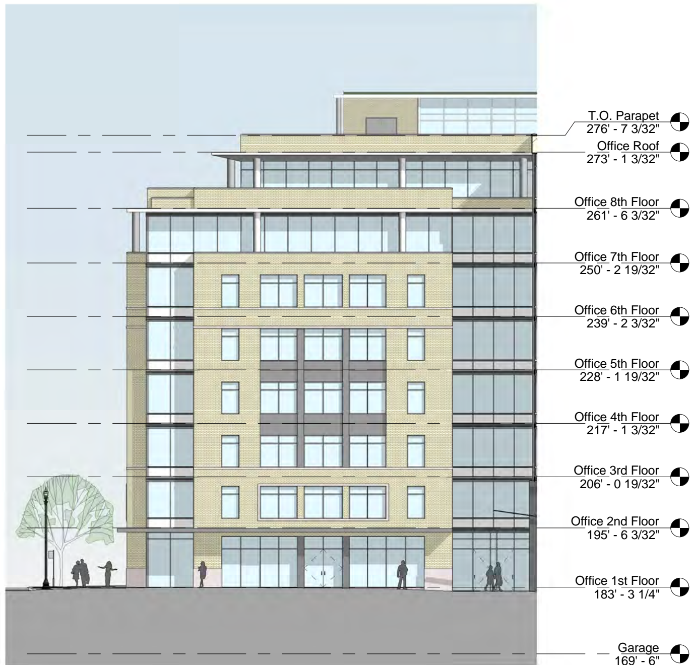
① Front Court East Elevation 1" = 20'-0"
