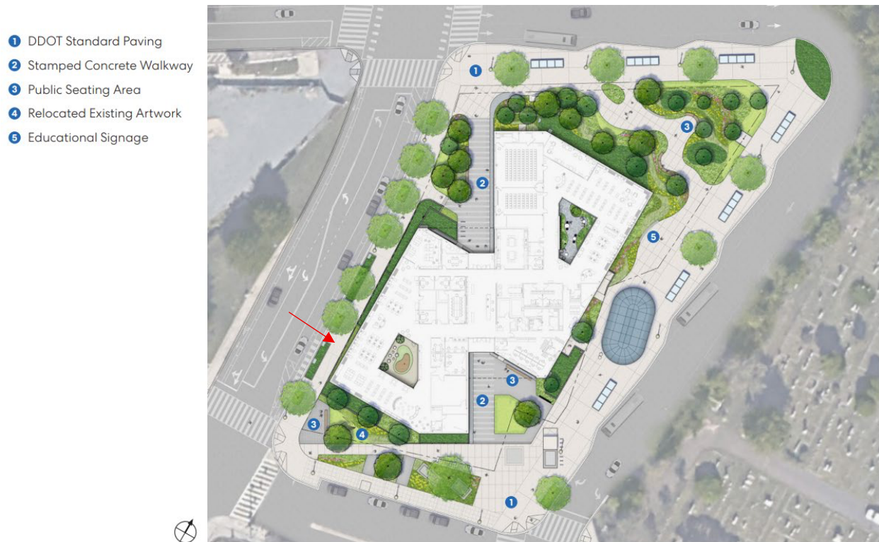
Figure 1: Library Illustrative Site Plan depicting where the building encroaches into the 10-foot front setback
