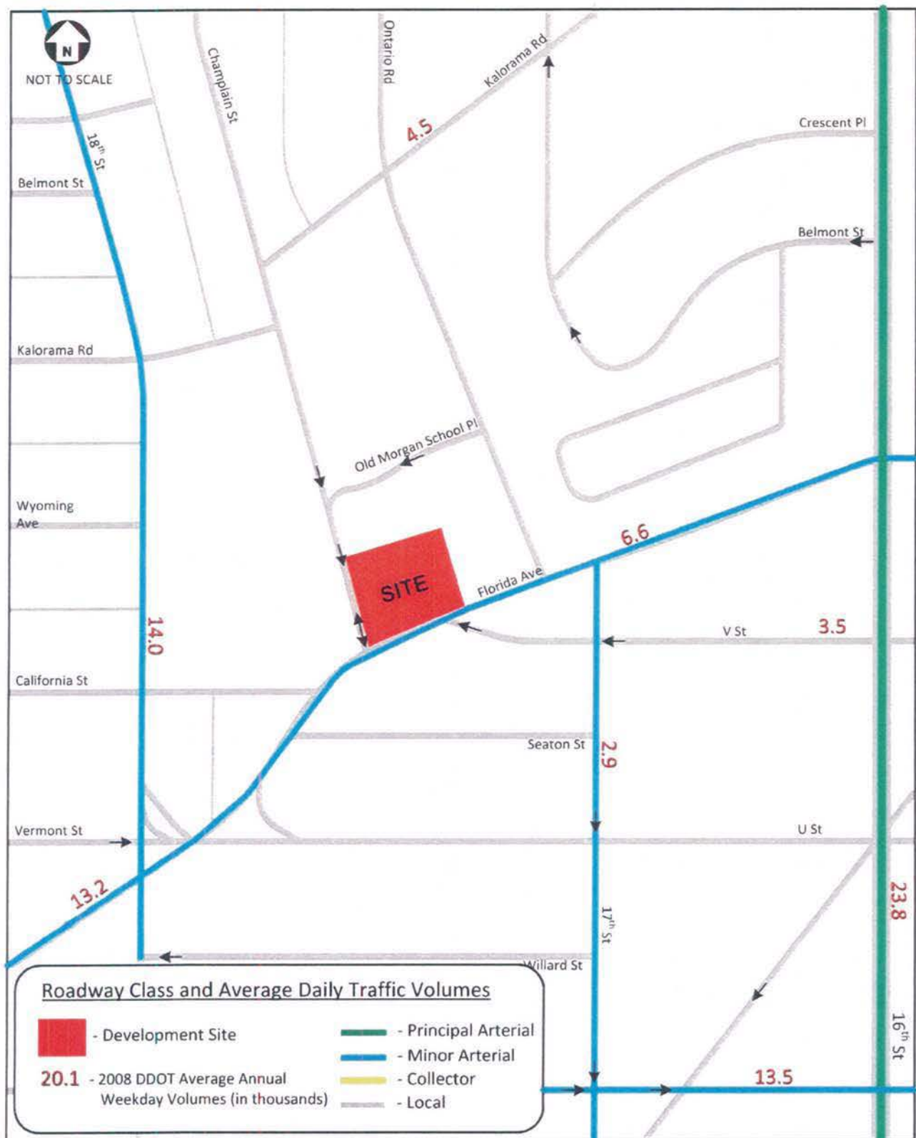
Figure 3: Roadway Classification and Average Daily Traffic
