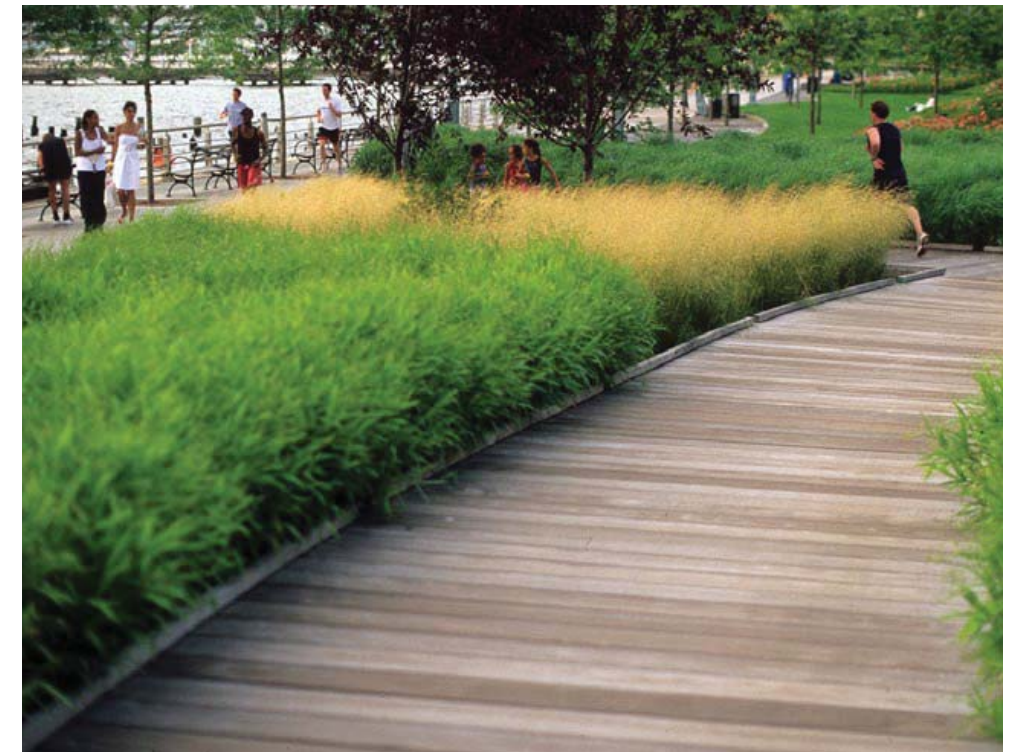
Kebony decking and bioretention planting
