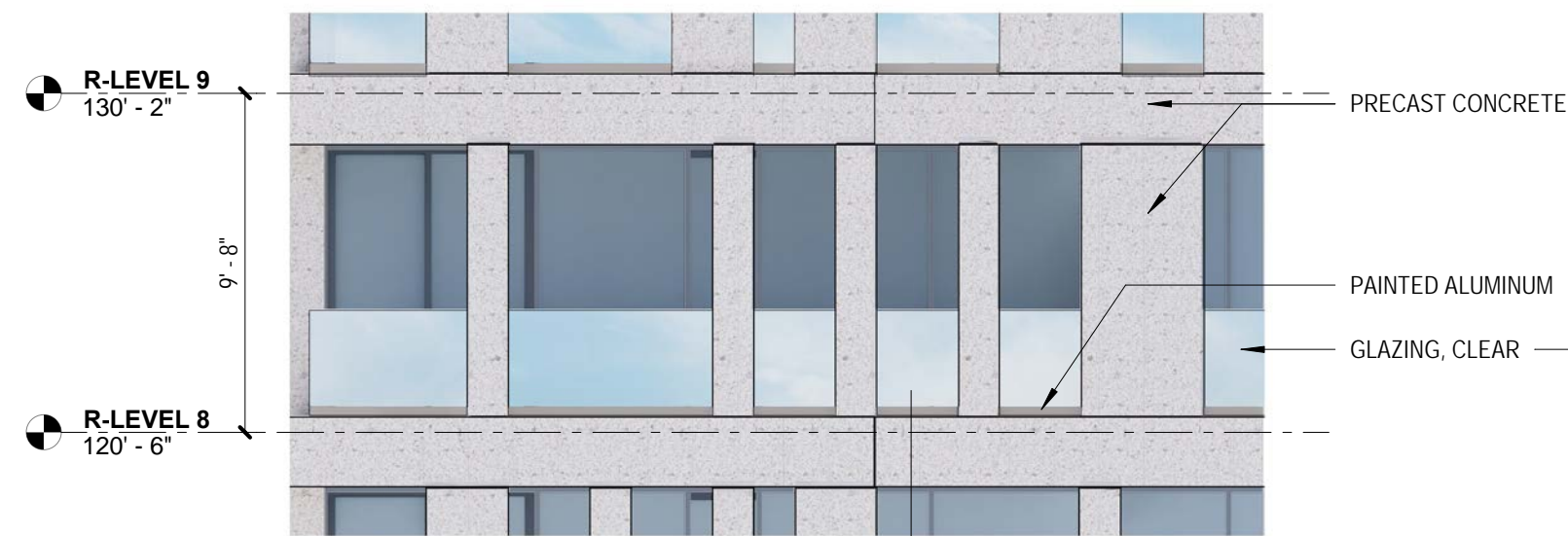
1a. ELEVATION AT BUILDING FACADE
