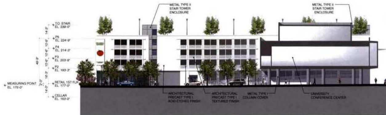
Approved Garage North Elevation
