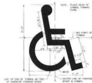
3 C-19 HANDICAP ACCESS STENCIL LAYOUT NOT TO SCALE
