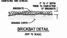
BRICKBAT DETAIL (NOT TO SCALE)
