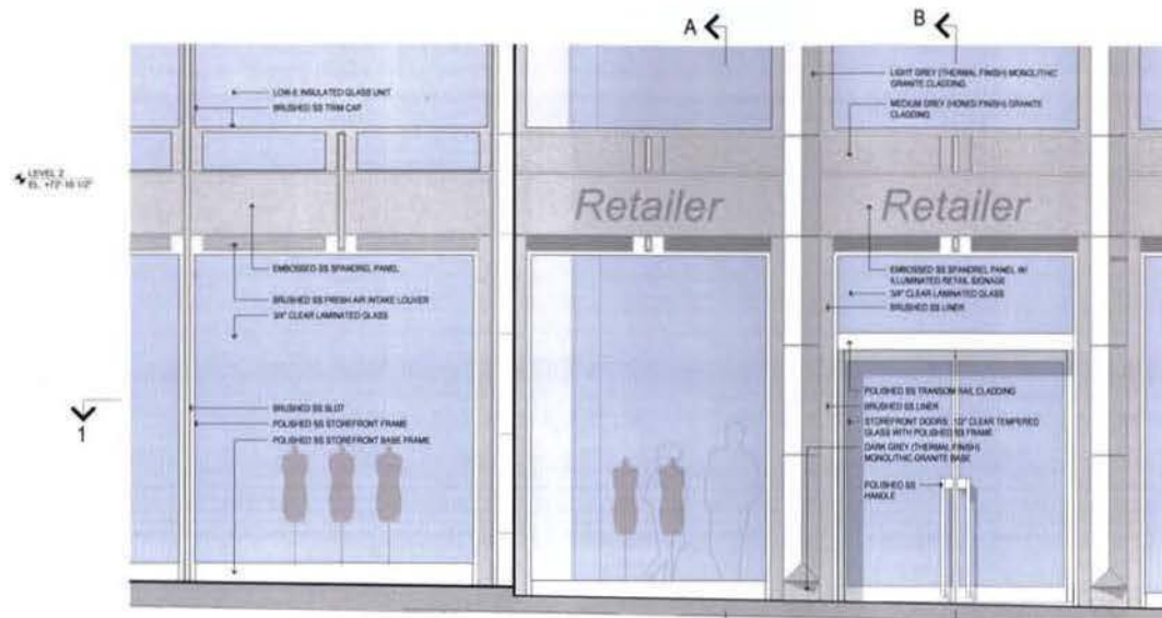
PARTIAL ELEVATION - K STREET
