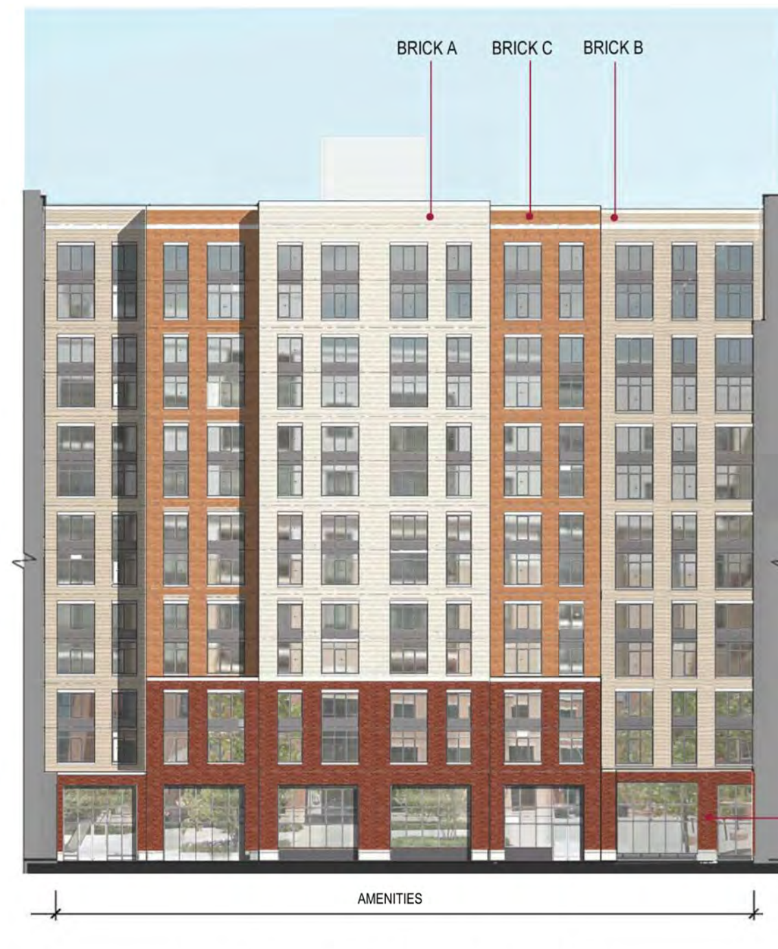
COURTYARD EAST ELEVATION
