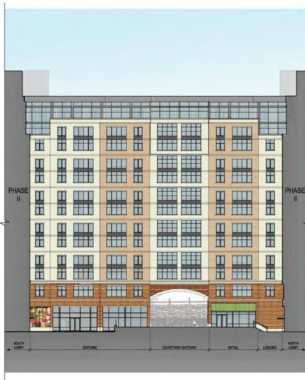
2 COURTYARD ELEVATION - COURTYARD GATEWAY SCALE: 1/32"=1'-0"
